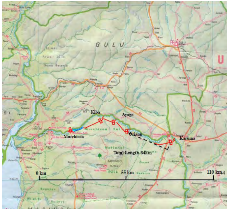
Figure 6.7.4-1 Transmission Line Route Map of Oriang Project
