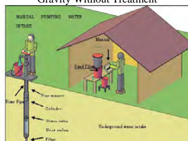
Manual Pumping Without Treatment
