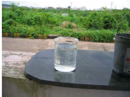
Treated effluent after chlorination
