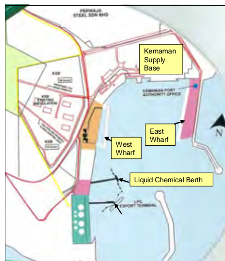
Figure 4.10-2 Layout of Terminals in Kemaman Port
