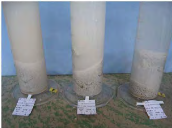
Photo-5 : Shaken 5 times (From right 30kg/m 3 , 60kg/m 3 , 90kg/m 3 cemented mixed per 1 m 3 of soil)
