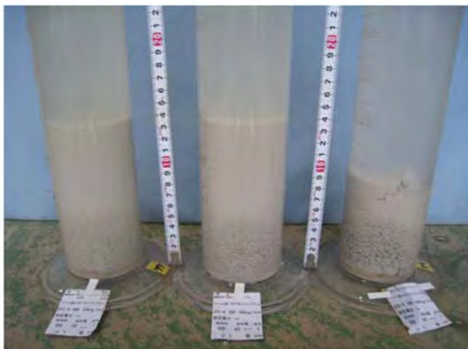
Photo-6 : Shaken 100 times (From right 30kg/m 3 , 60kg/m 3 , 90kg/m 3 cemented mixed per 1 m 3 of soil)
