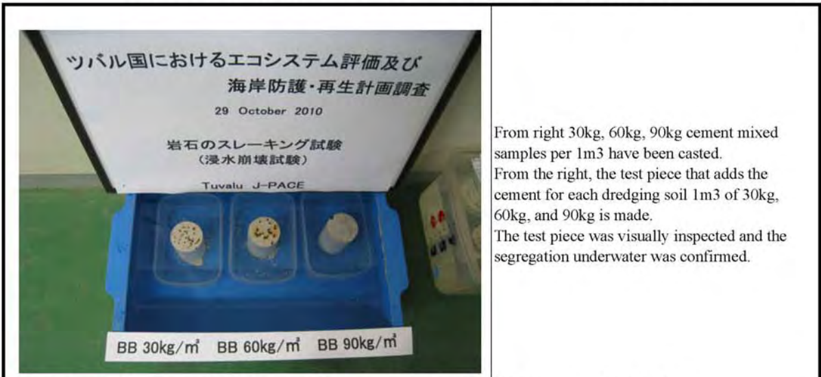
Photo-1 : Soaking Test of Soil Cemented Dredged Sand (At the Beginning of Soaking)
