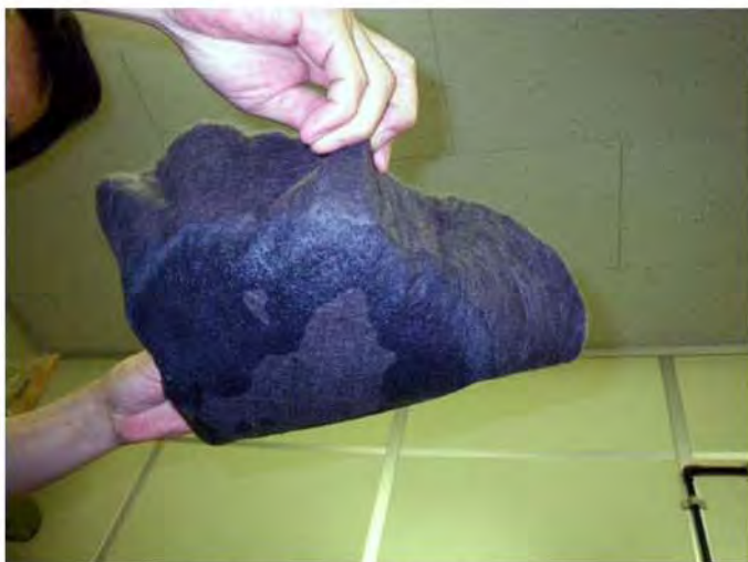
Photo-3 : Passing Through Test for Geofabric (5mm Thk. spun bond fabric) and Dredged Sand
