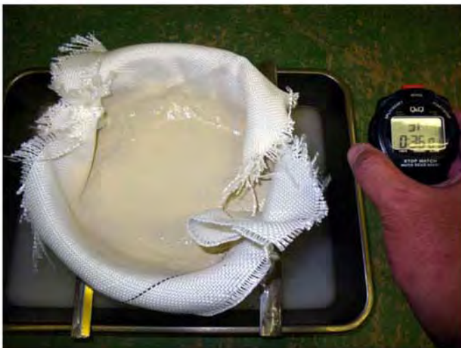
Photo-5 : Passing Through Test for Geofabric (1mm Thk. woven textile) and Dredged Sand
