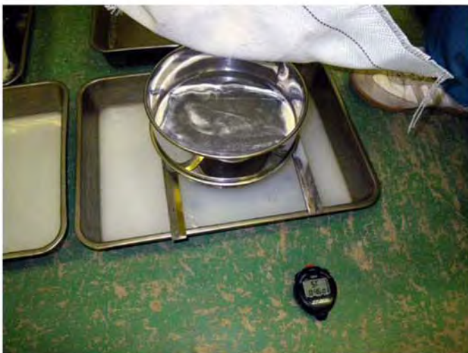
Photo-6 : Passing Through Test for Geofabric (1mm Thk. woven textile) and Dredged Sand
