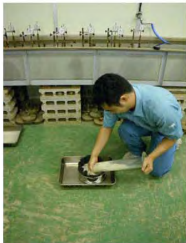
Photo-1 : Passing Through Test for Geofabric (5mm Thk. spun bond fabric) and Dredged Sand
