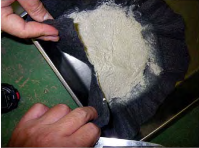
Photo-4 : Passing Through Test for Geofabric (5mm Thk. spun bond fabric) and Dredged Sand
