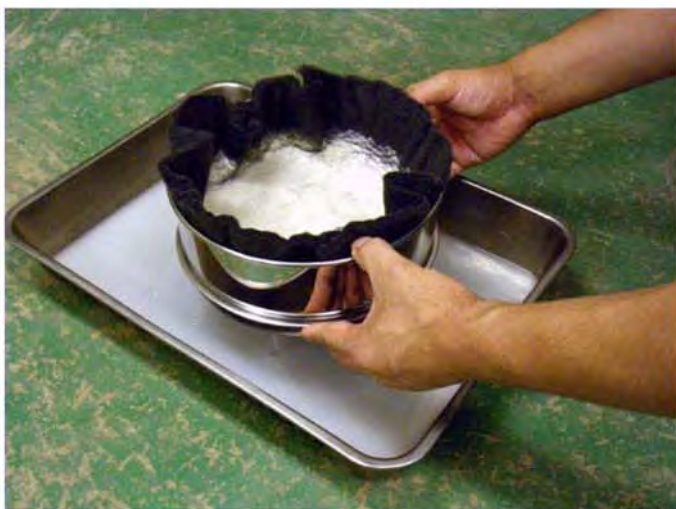
Photo-2 : Passing Through Test for Geofabric (5mm Thk. spun bond fabric) and Dredged Sand
