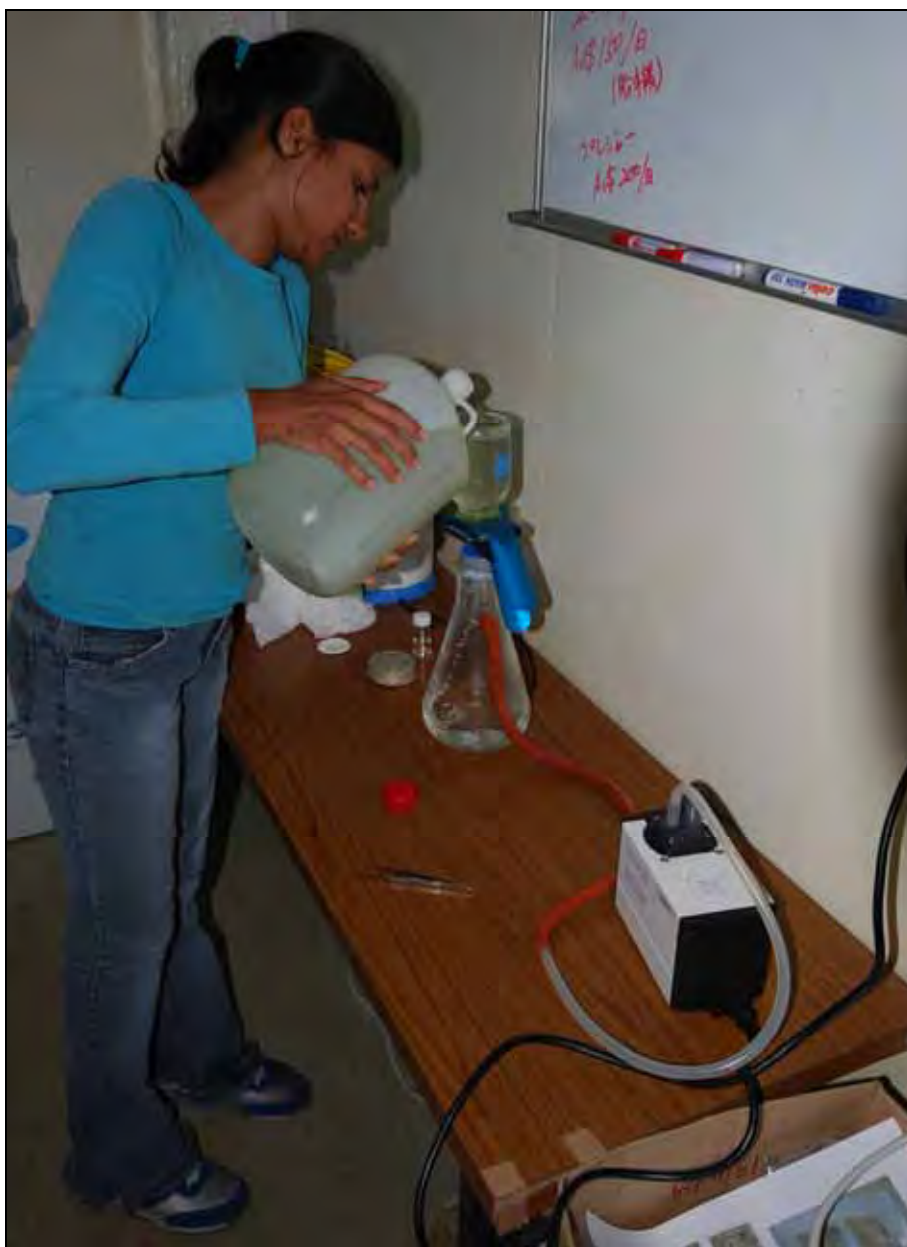
Figure 2.32 Water sample filtration procedure.
