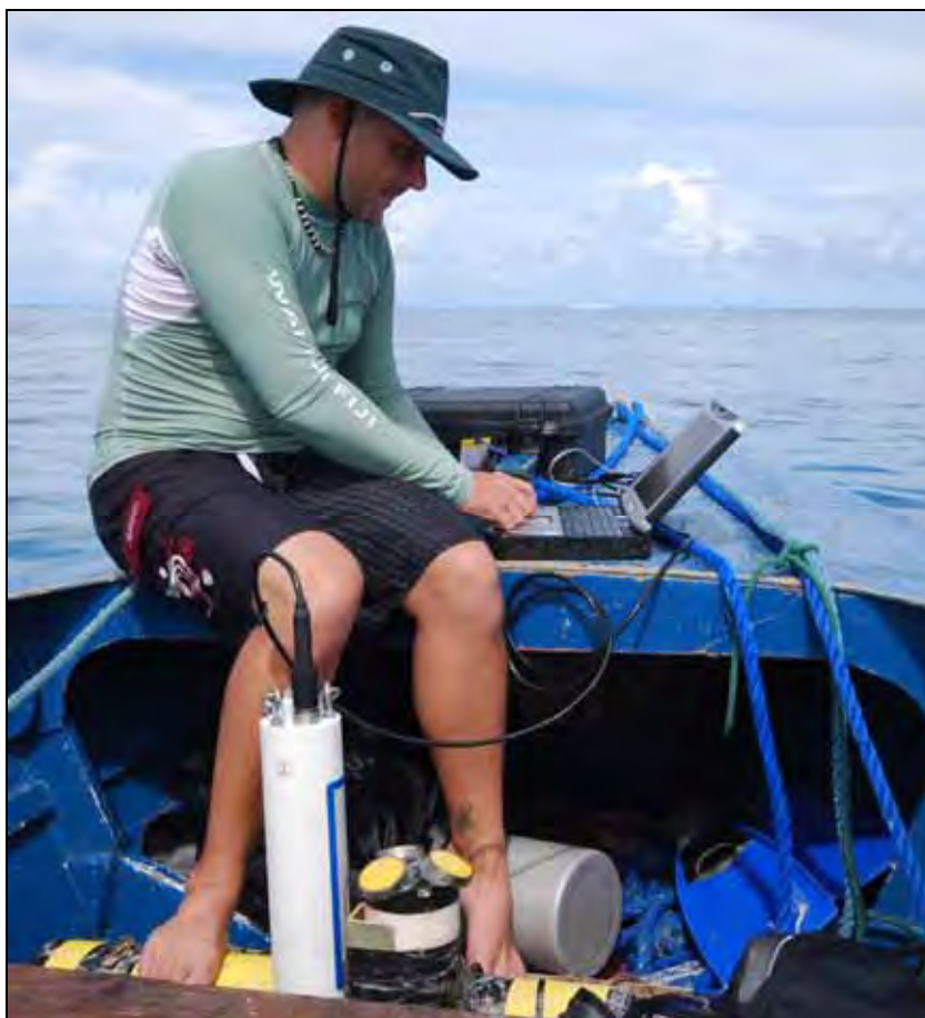
Figure 2.31 Hydrolab survey data download.
