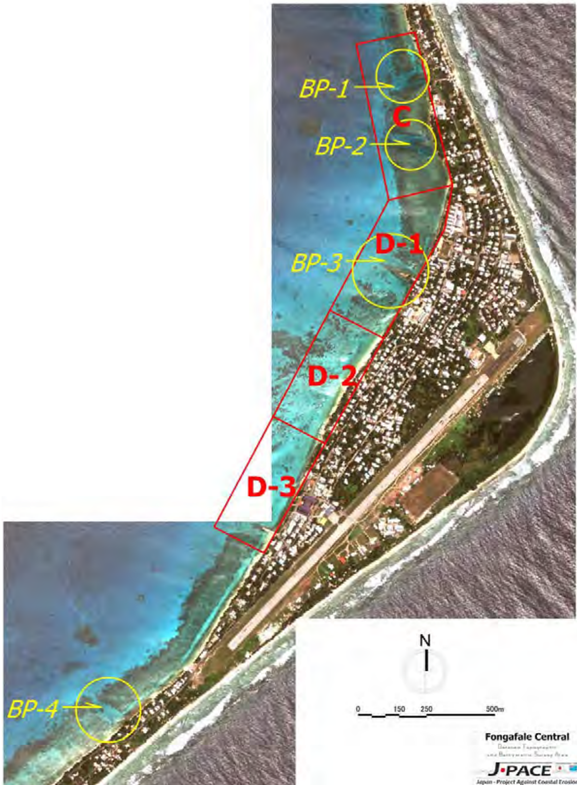
Figure 9.28 Detail Survey of Shallow Sea Area in the Target Zone for Coastal Protection Measures and Costal Borrow Pits
