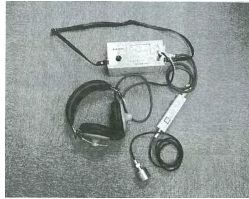
Photo-3 Electric Leakage Detector
