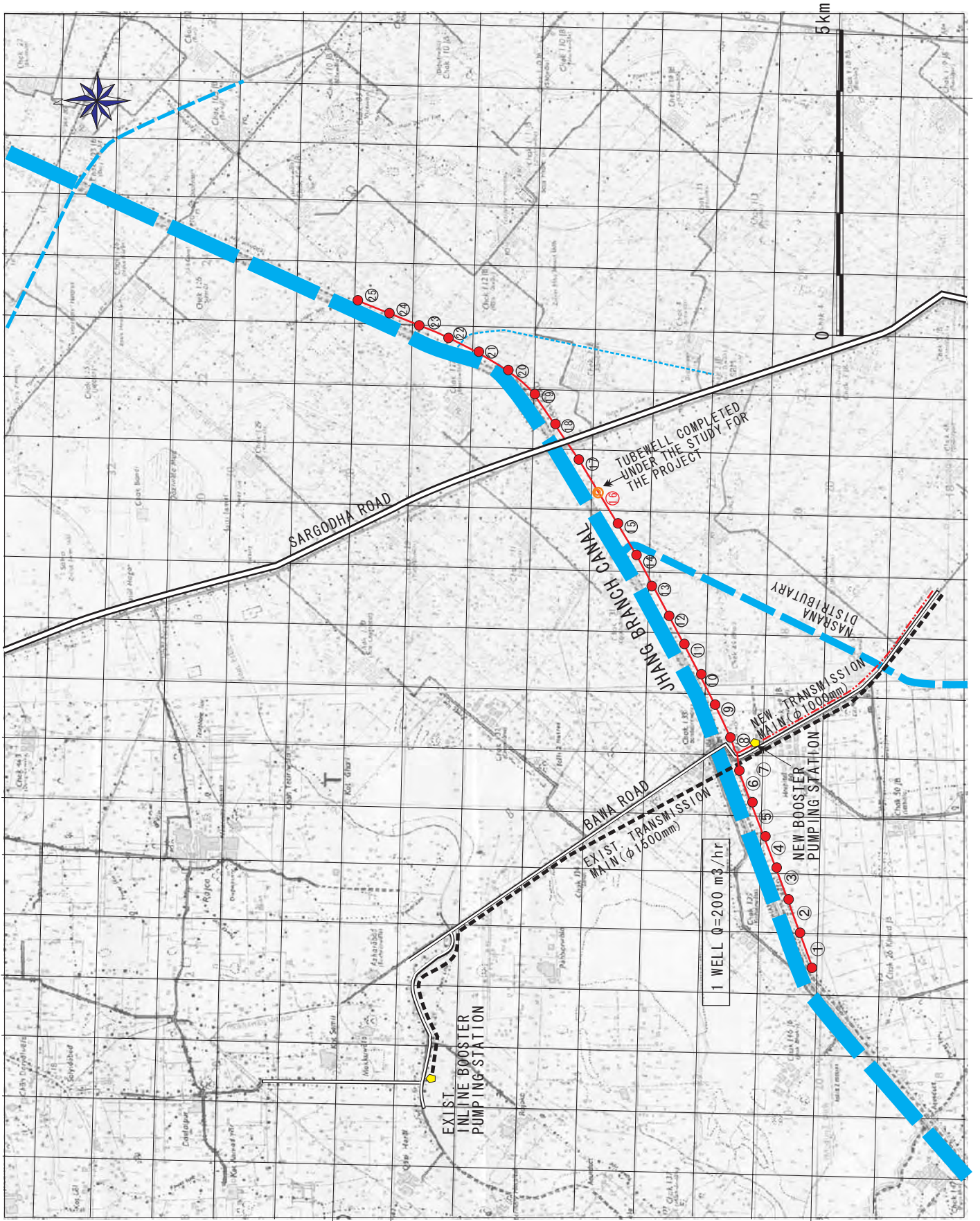
FIG. 2-10 LAYOUT OF TUBEWELLS ALONG JHANG BRANCH CANAL
