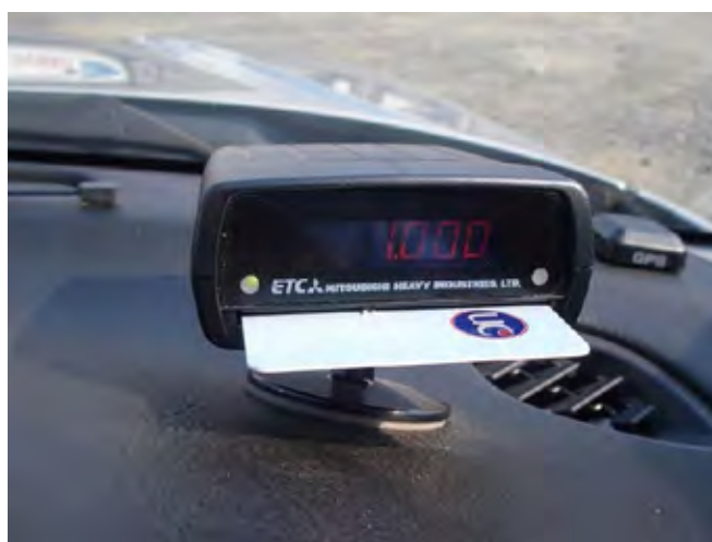
Figure 11.2 Active-DSRC On-Board-Unit (2-piece type)
