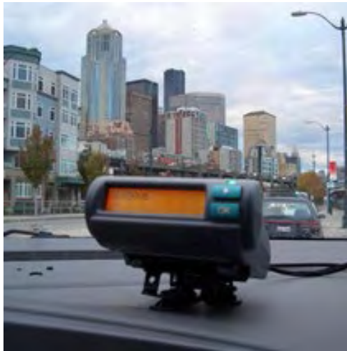
Figure 11.5 GPS / GSM On-Board-Unit
