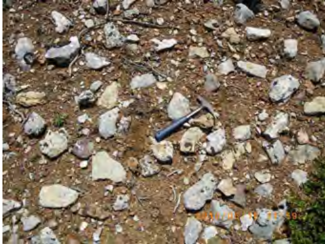
Gravelly soil distributes on the uneven ground surface. The material seemed to be transferred from upper reach by mudflow and consists of silty sand.
