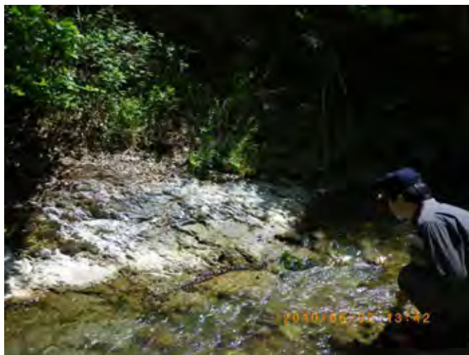
Photo 6 Mudstone cropped out at the riverbed of the upper dam site
