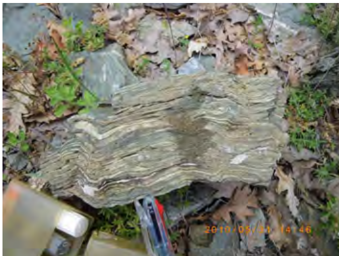
Photo 6 Some parts of the calcareous layer with a few mm thickness were dissolved
