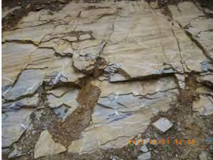
Splitting off in placibus along joints which intersect with schistosityes Photo 7 Schist distributed on the left bank slope of Gökçekaya reservoir
