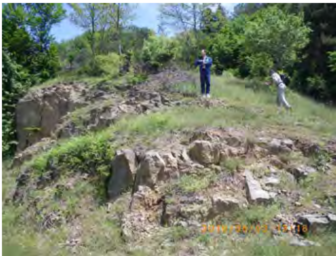
Photo 3 Sandstone cropped out on the slope of logging road at the right bank of Upper dam site
