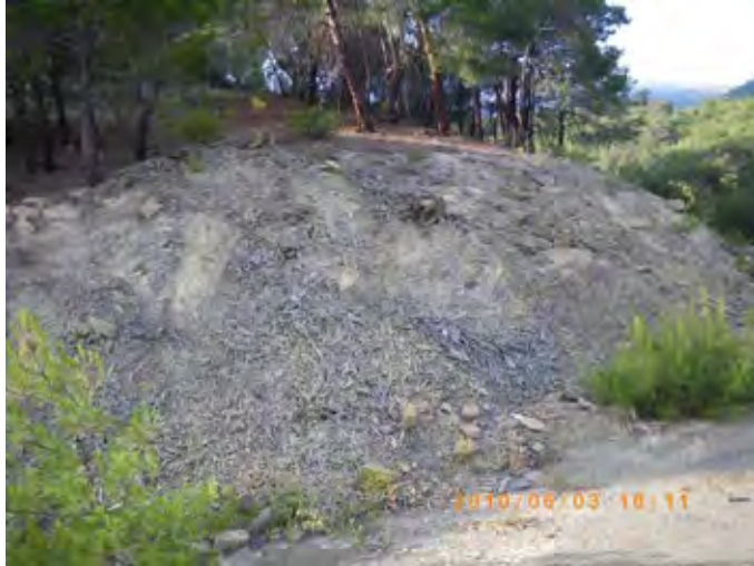
Photo 10 Mudstone cropped out at the outlet site, which is slaked by weathering
