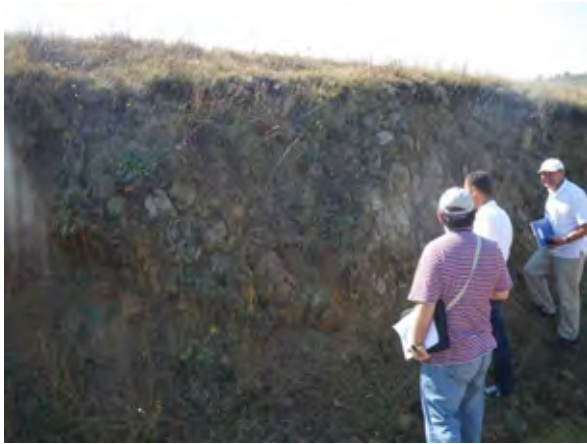
Photo 5.1 Tuff cropped out on the cut slope of the road around El.900m
