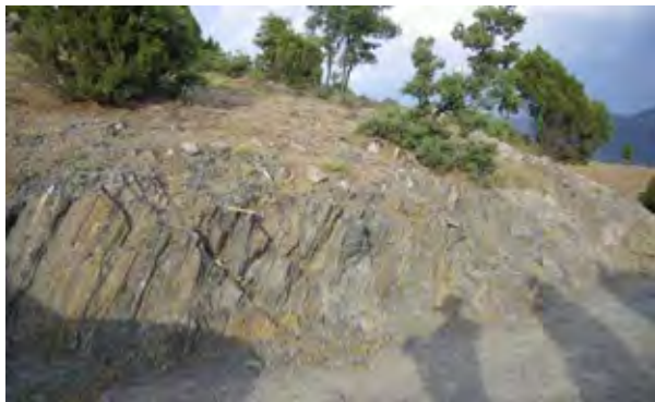
Photo 5.32 Outcrop of chlorite-biotite schist of PEg on the surface of headrace tunnel route
