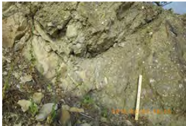
Photo 5.6 Sandstone (left) and conglomerate (right) crop out on the cut slope near the outlet site
