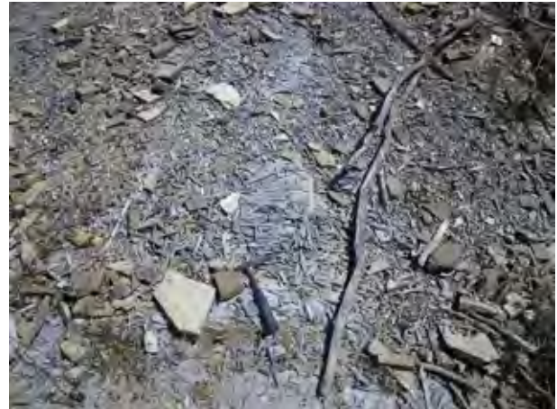
Photo 5.10 Crumbling mudstone to stick-like fragments by slaking
