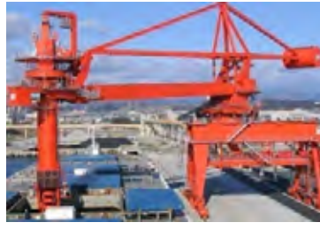
Unloader 1,400t/h, Height 43m
