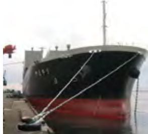
Domestic coal vessel "YAMAYURI": 12,000t, Length 140m, Width 26m, Self unloading type
