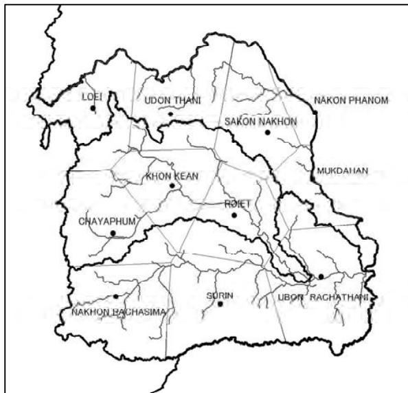
Thiessen polygon and TMD synoptic stations applied for Time-Series (Area Rainfall) Calculation
