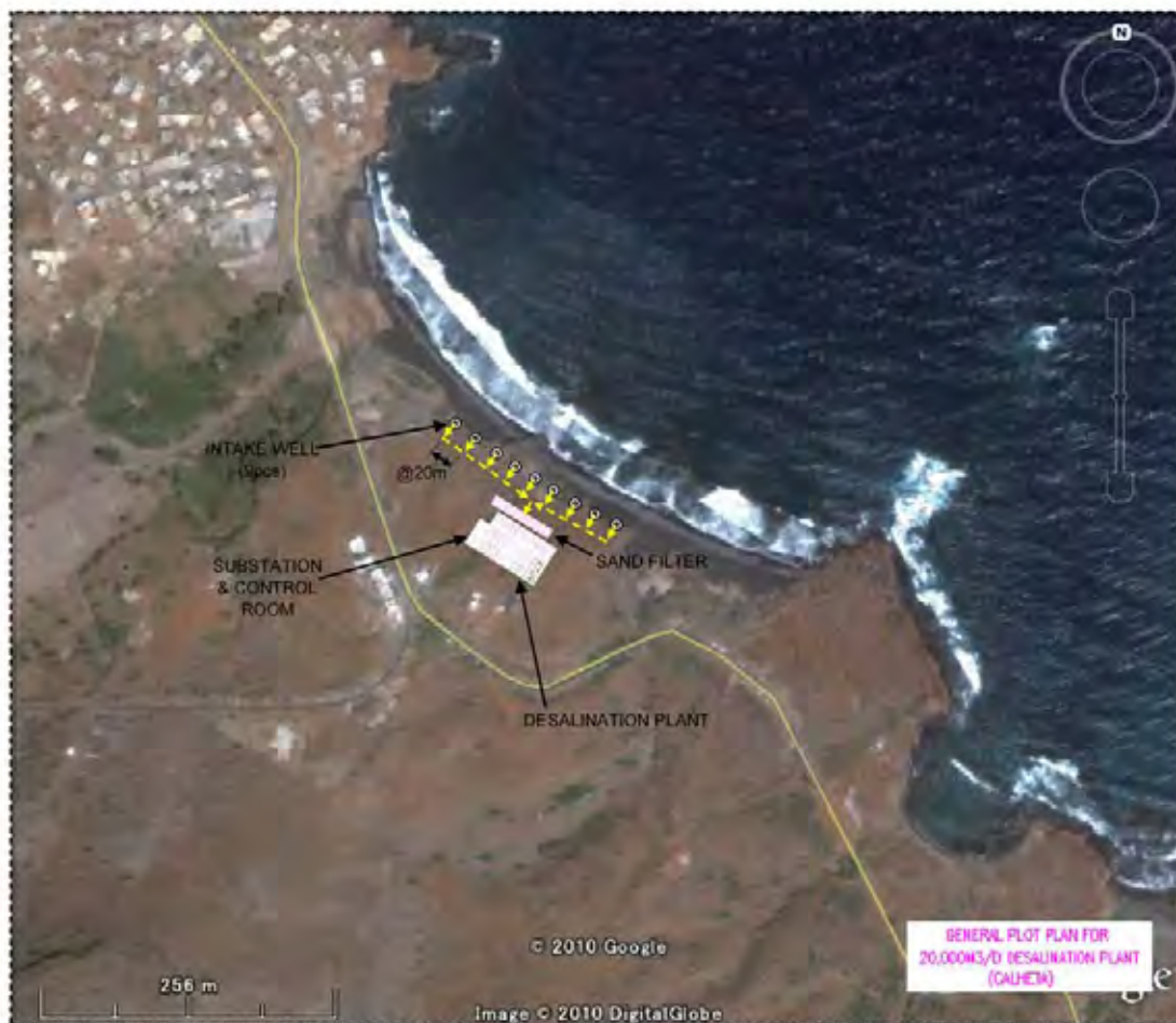
Figure 4.1-8: Sea Water Desalination Facility General Layout at Calheta
