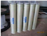
RO membrane 8 inch dia x 40 inch length SW30HR-370 (DOW) 7 elements are loaded in 1 PV.
