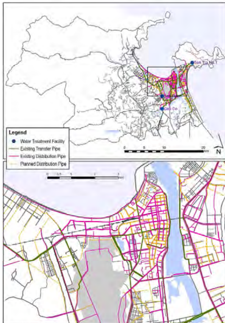
Figure 8.3.2 Water Pipeline Network in Danang City
