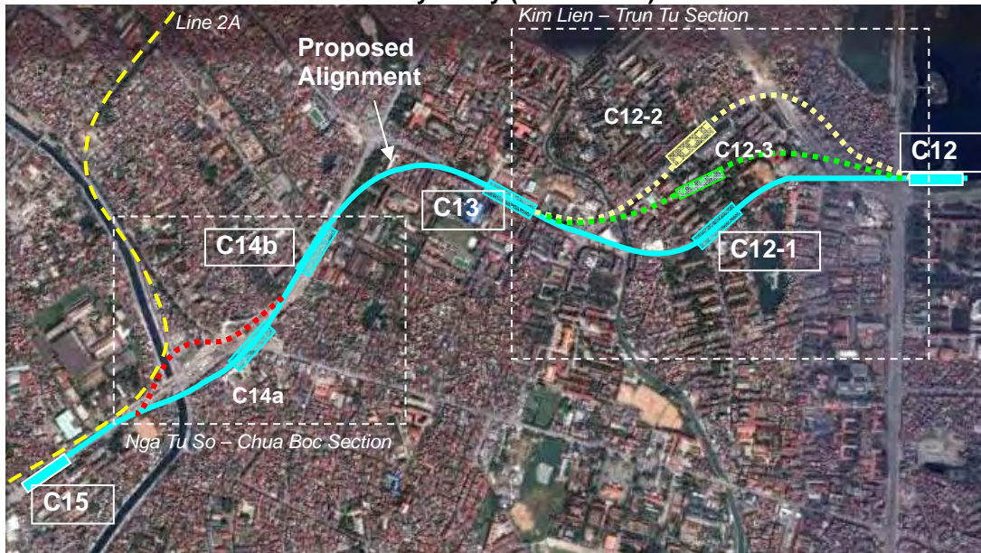
Figure 4.1.16 Alternatives for Alignment and Station Locations of Phase2 section in the Feasibility Study (TEDI South)
