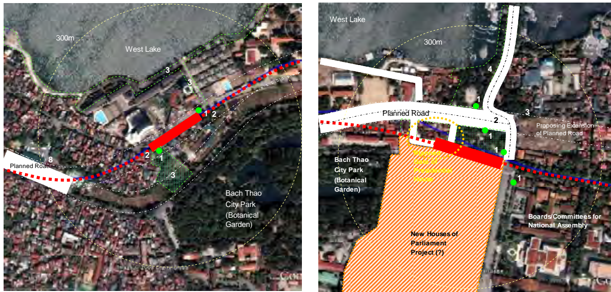
Figure 4.1.14 Necessary Alignment Conformity with UMRT Line2 and New Road Scheme along West Lake to fix locations of Bach Khoa Station (C6) and Ho Tay Station (C7)
