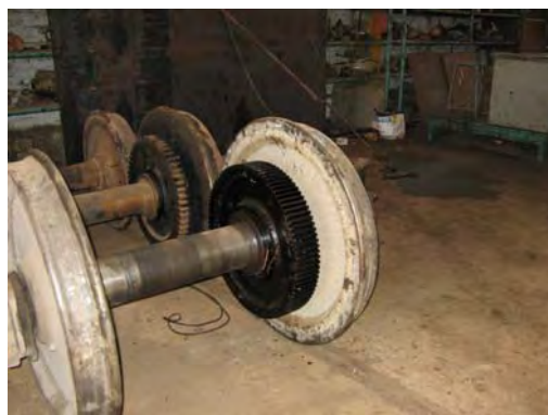
Excessively worn locomotive wheel
