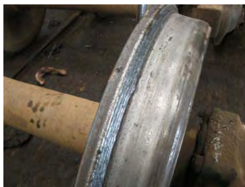
Welded frange to be cut by wheel lathe
