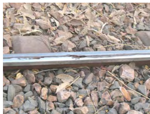
Longitudinal crack of rail
