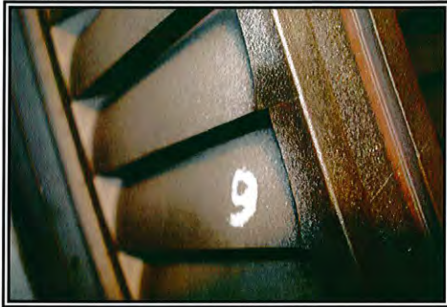
Photo 9 IP Rotating Blade – Surface Roughness of 9 th Stage
