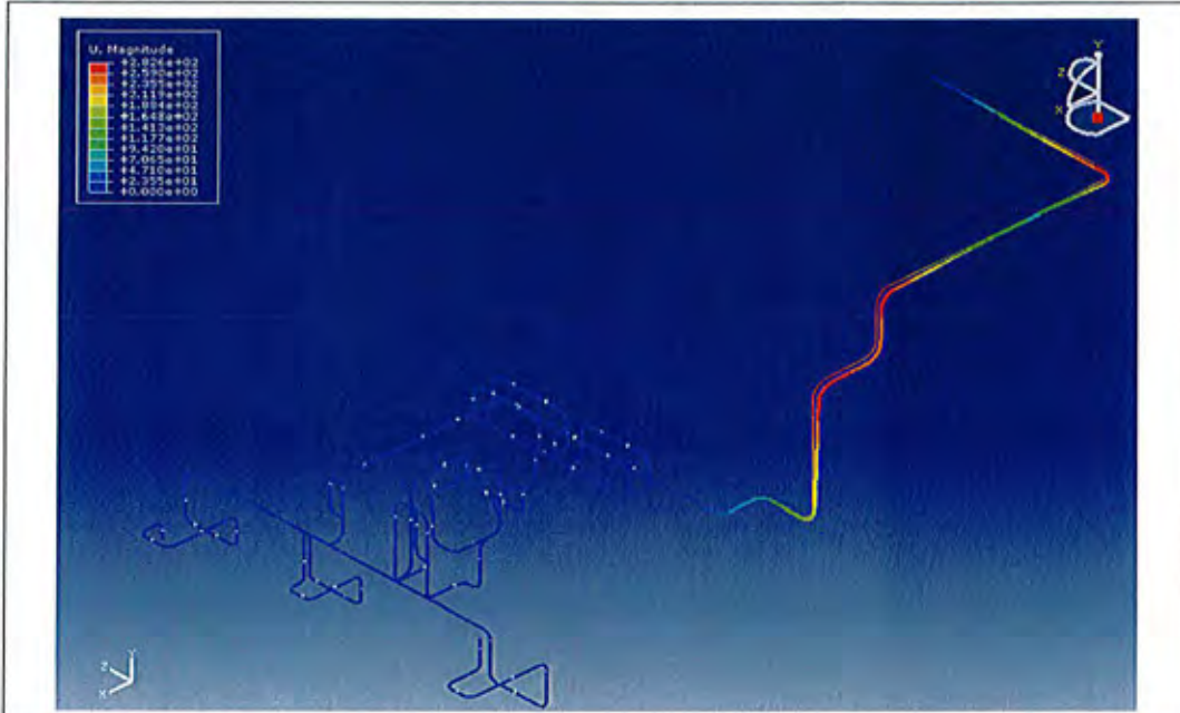
Figure 12.6: Deflection Plot – Hot position superimposed plot showing deformed and undeformed plot. (View scaled by 2 times)
