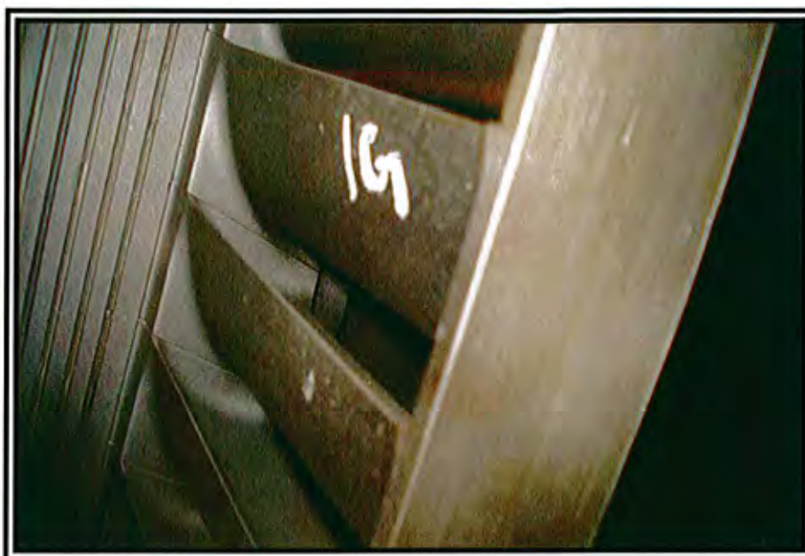
Photo 15 LP Rotating Blade – Surface Roughness of 1 st Stage
