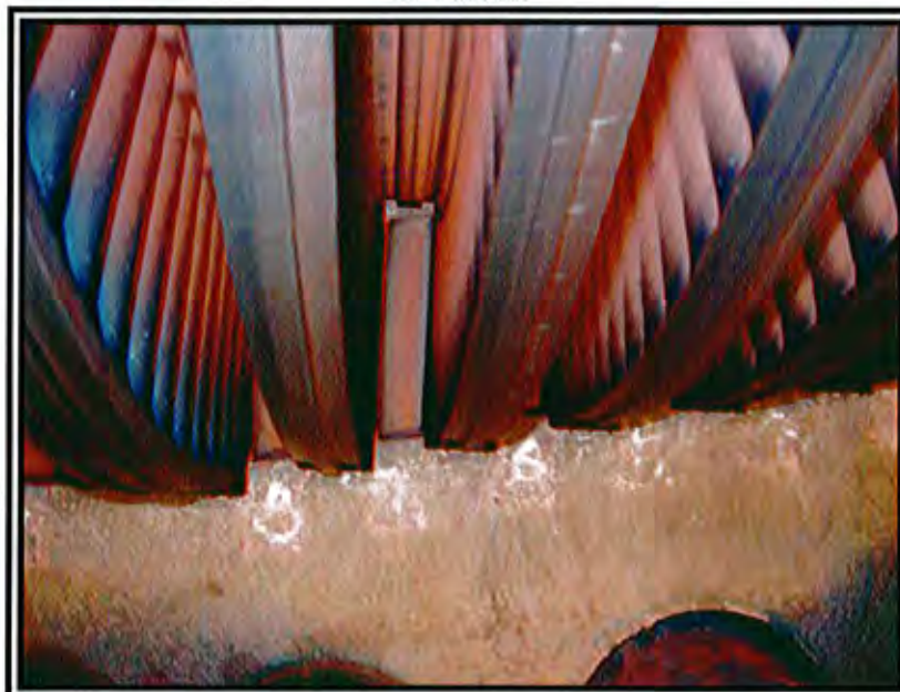
Photo 20 IP-Interstage packing 5 th stage
