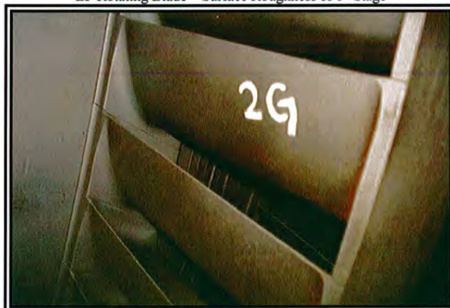
Photo 16 LP Rotating Blade – Surface Roughness of 2 nd Stage
