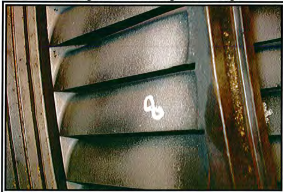
Photo 8 IP Rotating Blade – Surface Roughness of 8 th Stage
