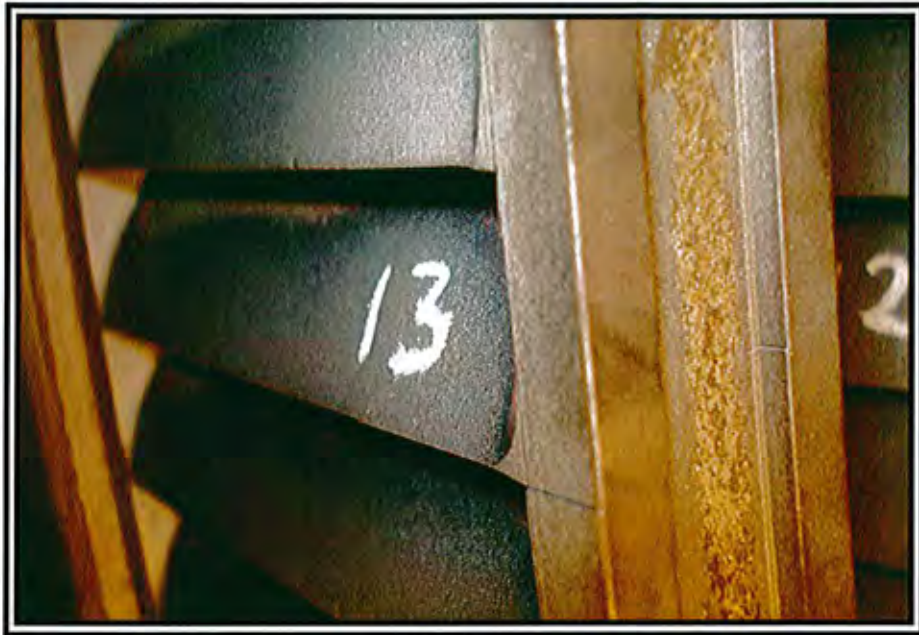
Photo 13 IP Rotating Blade – Surface Roughness of 13 th Stage
