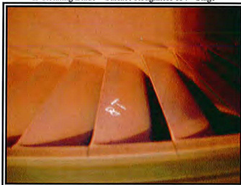
Photo 8 IP Rotating Blade – Surface Roughness of 8 th Stage
