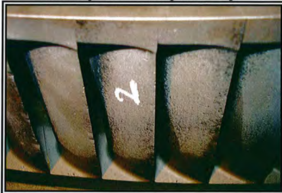
Photo 2 IP Rotating Blade – Surface Roughness of 2 nd Stage
