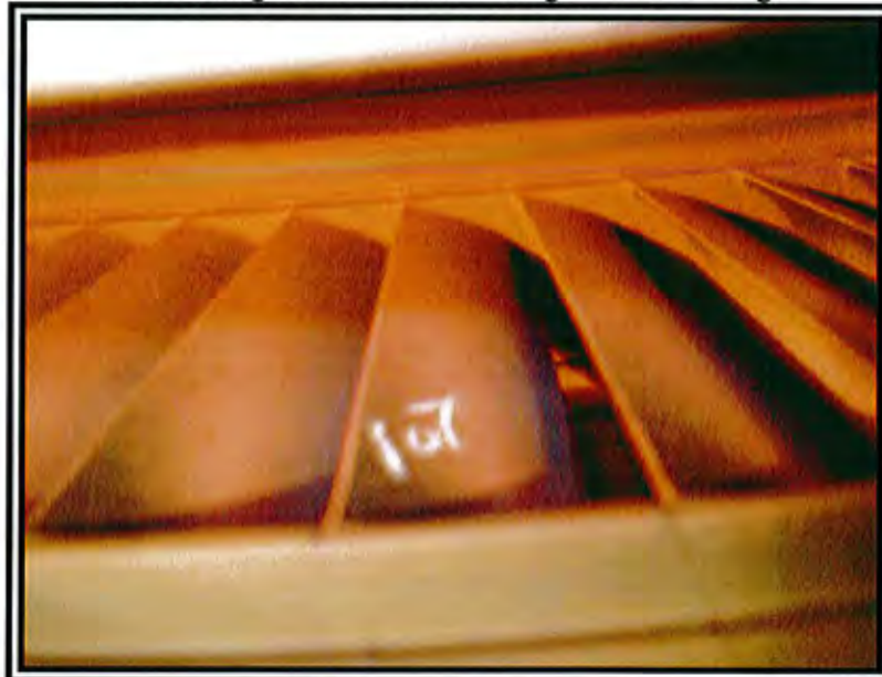
Photo 10 IP Rotating Blade – Surface Roughness of 10 th Stage
