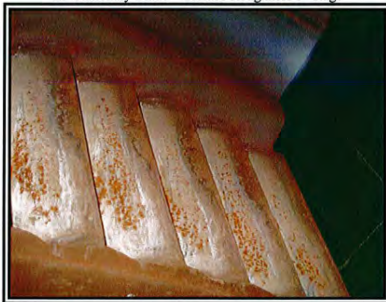
Photo-24 LP Stationary Blade – Surface Roughness
