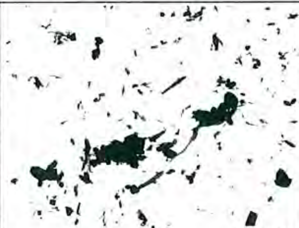
Fine granular and needlelike precipitates disappeared
