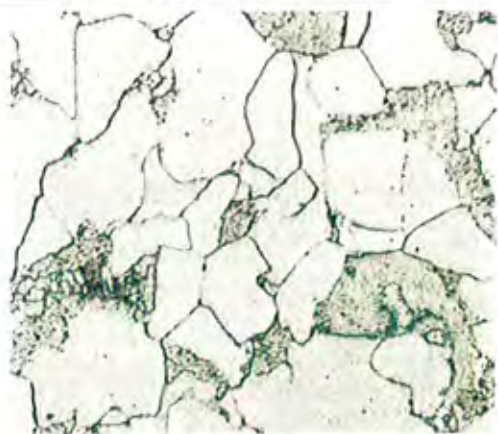
Rod-shaped precipitates in ferrite grain slightly appeared
