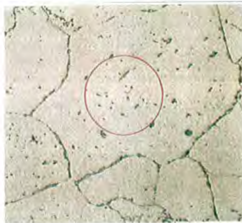
Rod-shaped precipitates in ferrite grain remarkably appeared
