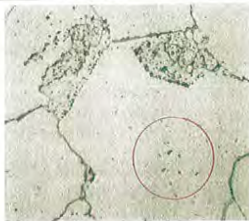
Rod-shaped precipitates in ferrite grain slightly appeared
