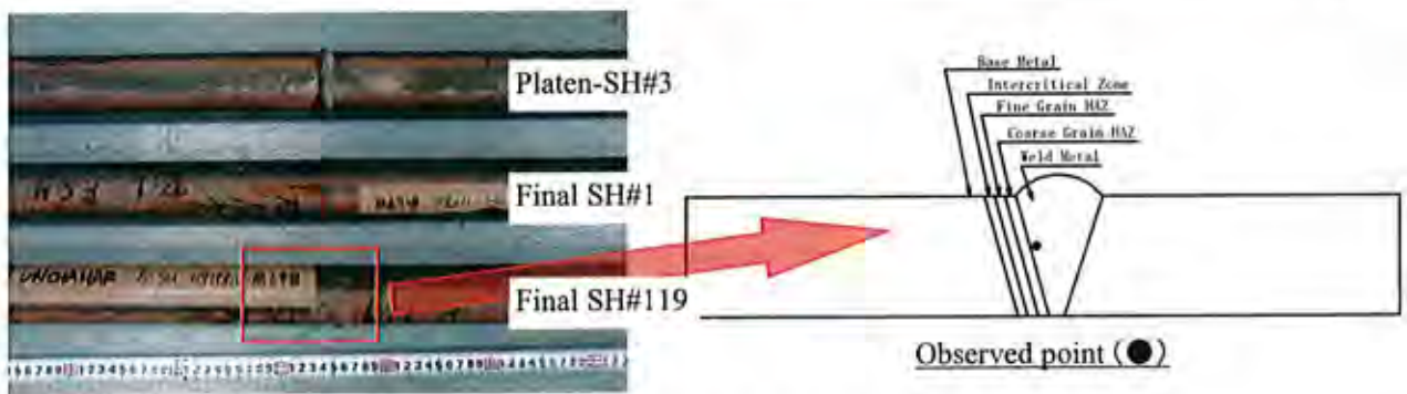
Photo II -54 Microstructure observation at cross section of sample tube [Final-SH #119 (Weld Metal) ]
