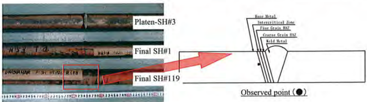
Photo II -50 Microstructure observation at cross section of sample tube [Final-SH #119 (Base Metal) ]
