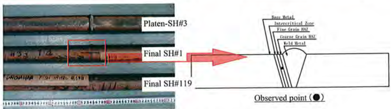
Photo II -41 Microstructure observation at cross section of sample tube [Final-SH #1 (Fine Grain HAZ) ]
