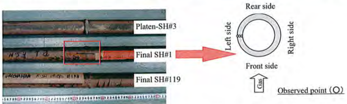
Photo II -25 Microstructure observation at cross section of sample tube [ Final-SH #1 (left side, Base Metal) ]
