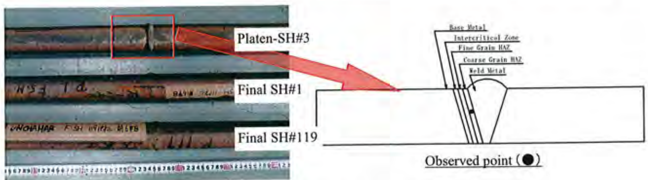
Photo II -31 Microstructure observation at cross section of sample tube [Platen-SH#3 (Coarse Grain HAZ) ]
