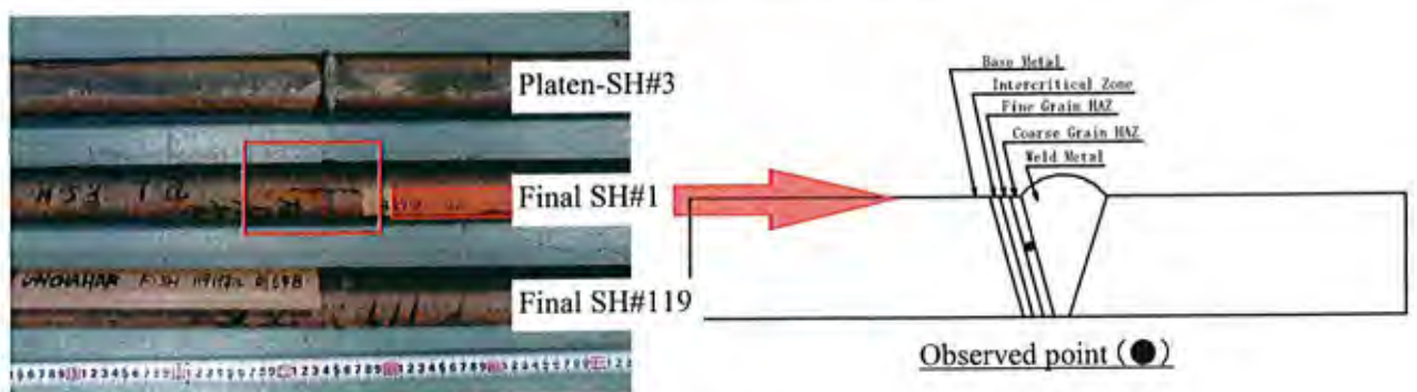
Photo II -42 Microstructure observation at cross section of sample tube [Final-SH #1 (Coarse Grain HAZ) ]
