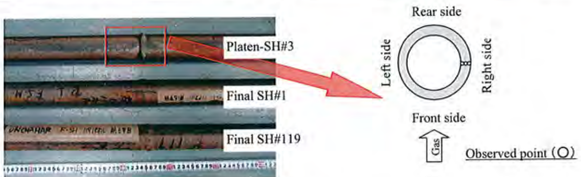
Photo II -22 Microstructure observation at cross section of sample tube [Platen-SH#3 (right side, Base Metal) ]
