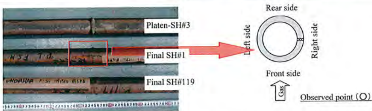
Photo II -24 Microstructure observation at cross section of sample tube [Final-SH #1 (right side, Base Metal) ]
