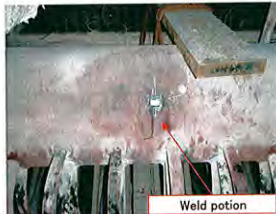
Measurement point of right side of RH outlet header
