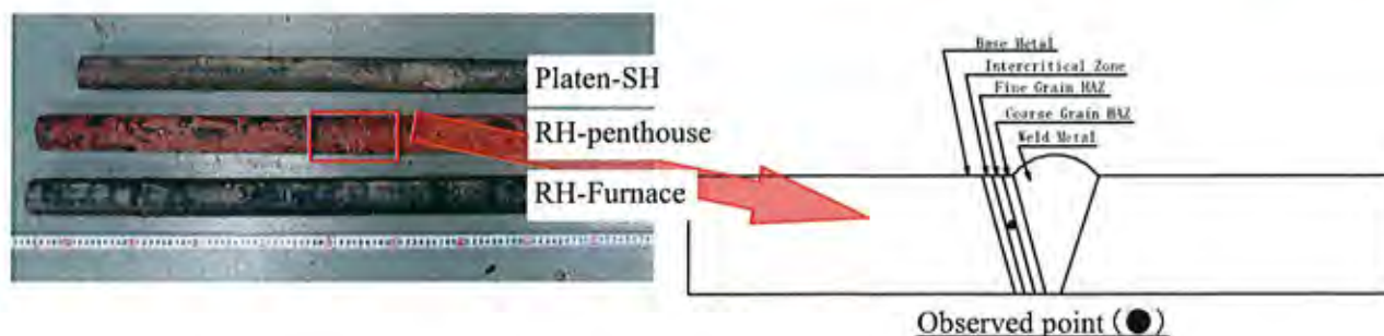
Photo I -39 Microstructure observation at cross section of sample tube [RH-Penthouse (Fine Grain HAZ) ]
