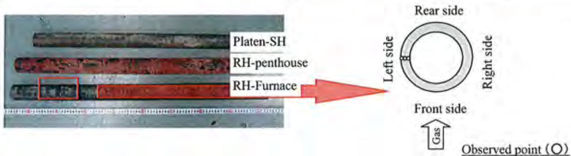
Photo I -25 Microstructure observation at cross section of sample tube [RH-Furnace (left side, Base Metal) ]
