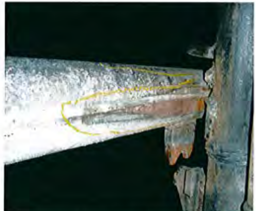
Thinning portion of cooling spacer tube
