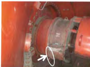
Photo-3: LP turbine packingland Turbine side (Lower/Left)
