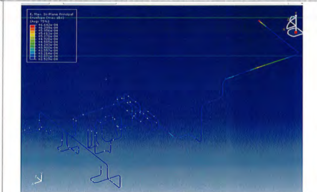
Figure 12.7: Elastic strain Plot – Hot position (Max 0.00066)
