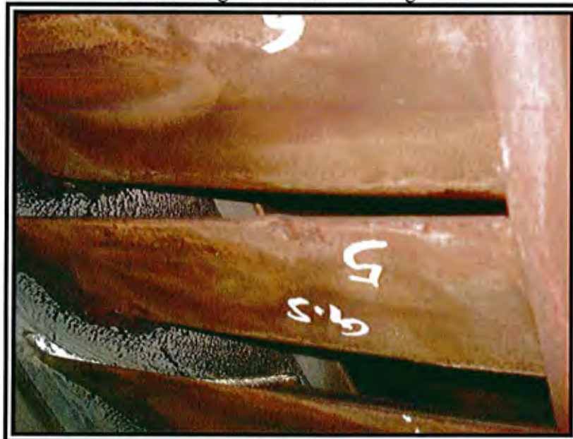
Photo-22 LP Stationary Blade – Surface Roughness 5 th stage
