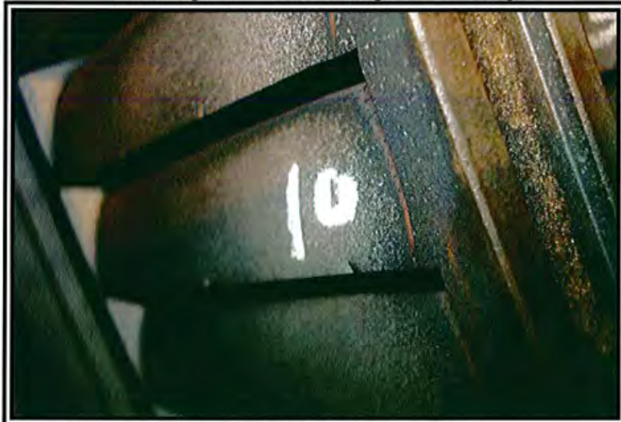
Photo 10 IP Rotating Blade – Surface Roughness of 10 th Stage
