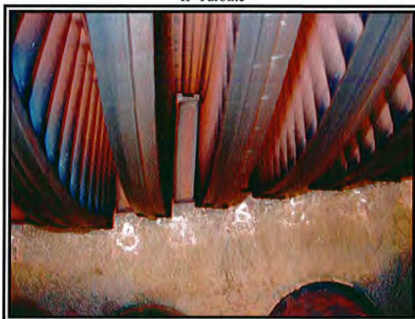
Photo 20 IP-Interstage packing 5 th stage
