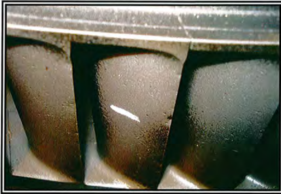
Photo 1 IP Rotating Blade – Surface Roughness of 1 st Stage
