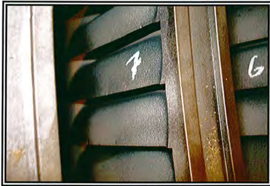
Photo 7 IP Rotating Blade – Surface Roughness of 7 th Stage
