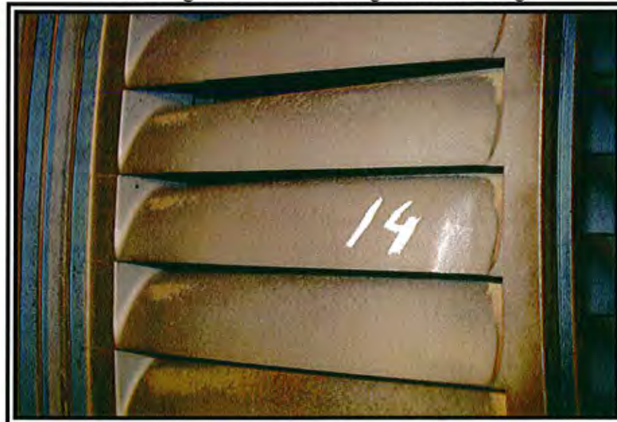
Photo 14 IP Rotating Blade – Surface Roughness of 14 th Stage
