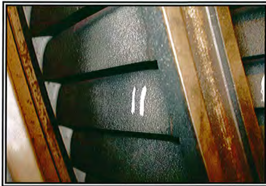
Photo 11 IP Rotating Blade – Surface Roughness of 11 th Stage
