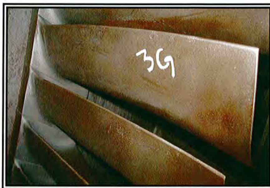
Photo 17 LP Rotating Blade – Surface Roughness of 3 rd Stage
