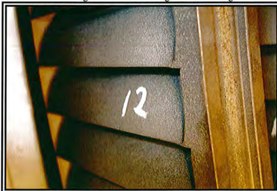
Photo 12 IP Rotating Blade – Surface Roughness of 12 th Stage
