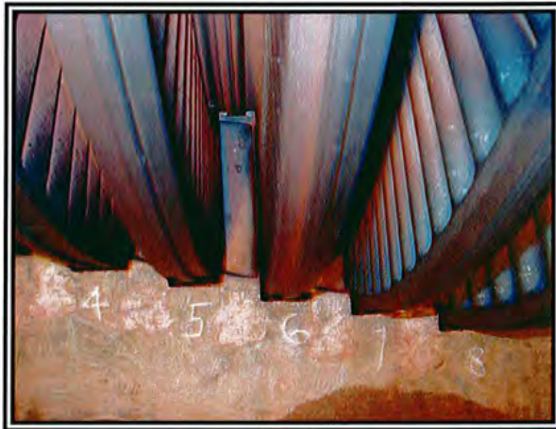
Photo 17 IP –Condition of Tip spill strip in 4 th , 5 th , 6 th & 7 th stage
