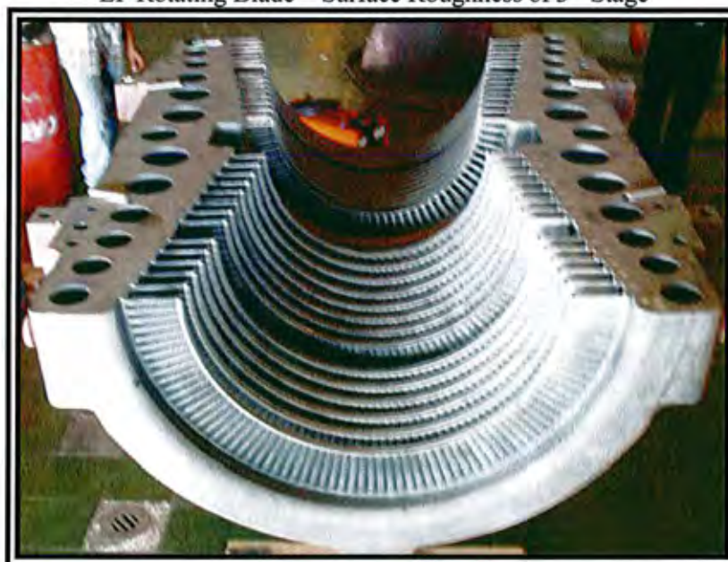
Photo 18 IP bottom Casing - after Sand Blasting
