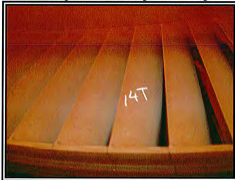
Photo 14 IP Rotating Blade – Surface Roughness of 14 th Stage
