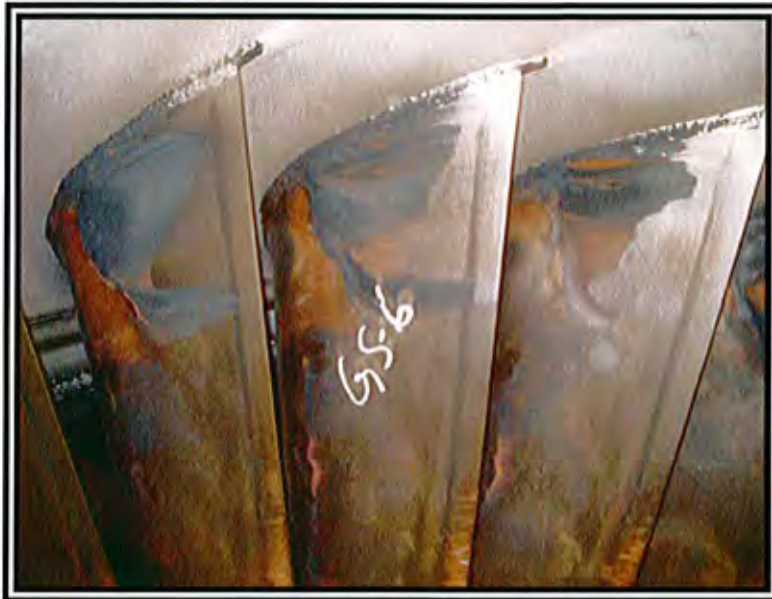
Photo-23 LP Stationary Blade – Surface Roughness 6 th stage
