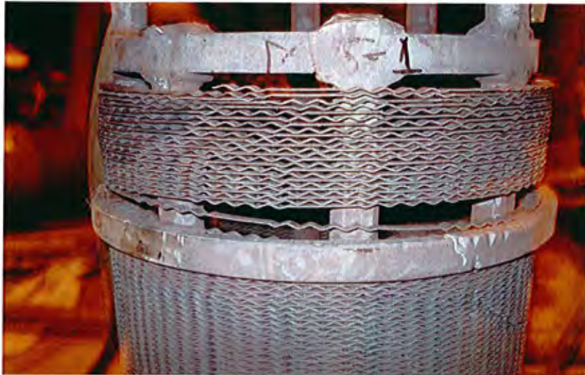
The view of damage body of strainer MS -1.
