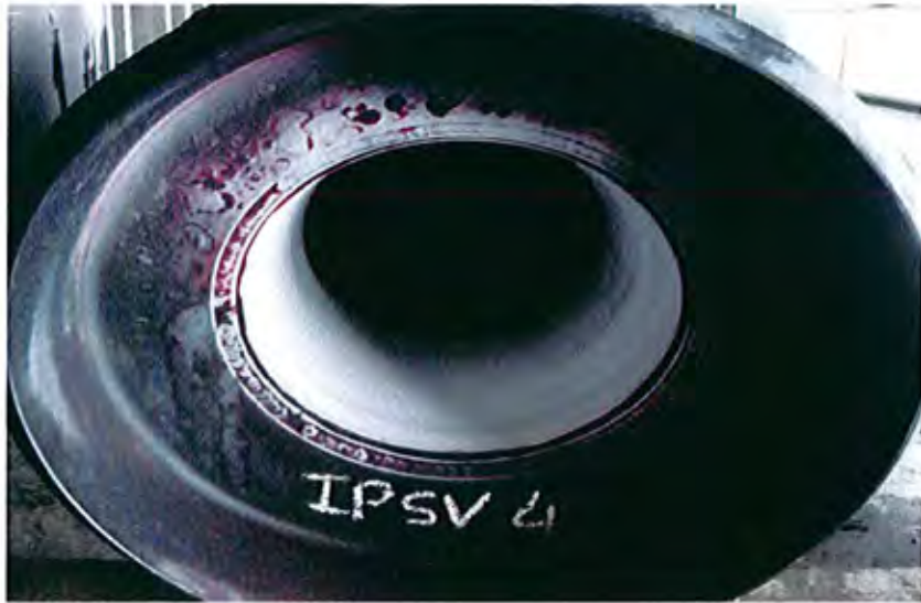
The view of LPT test on IP SV -4
