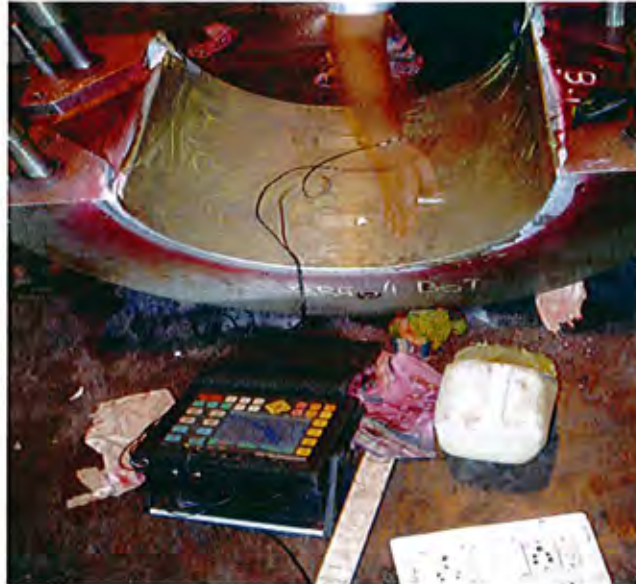
The photograph of UT on bearing.
