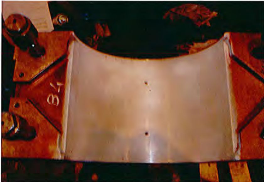
The view of LPT on bottom bearing no 4
