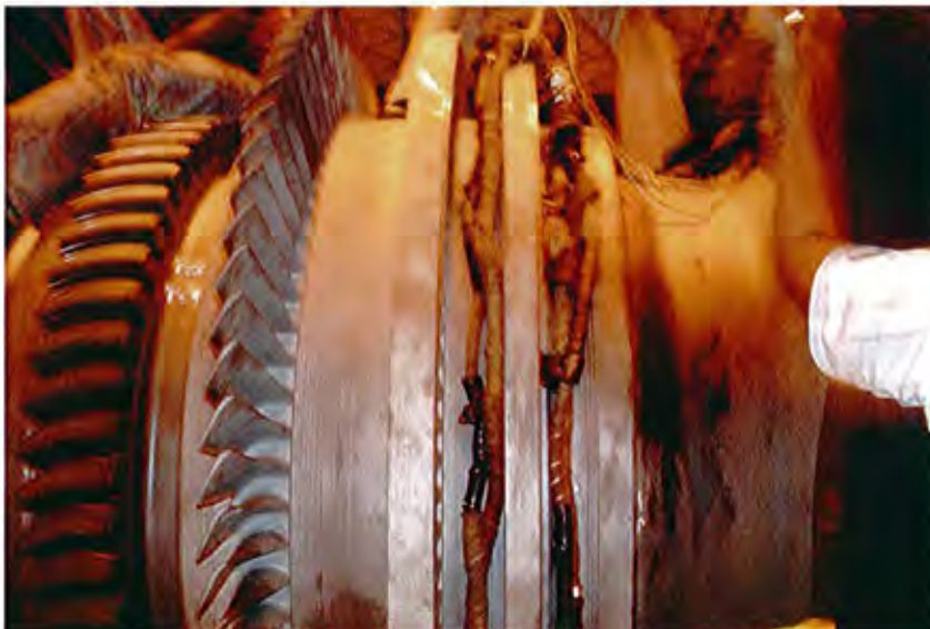
The photograph of Coil MPI testing on LP rotor.
