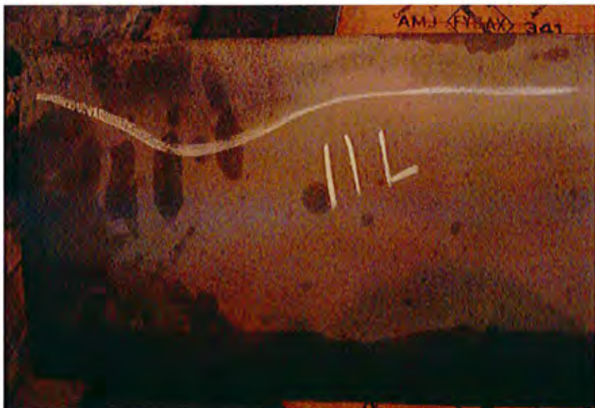
The steam erosion observed on blade of LP rotor.
