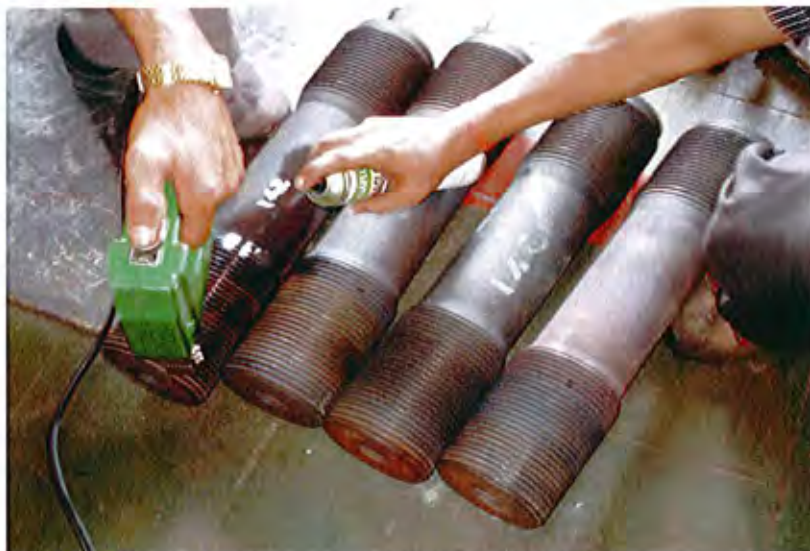
The view of MPI on LP casing studs.
