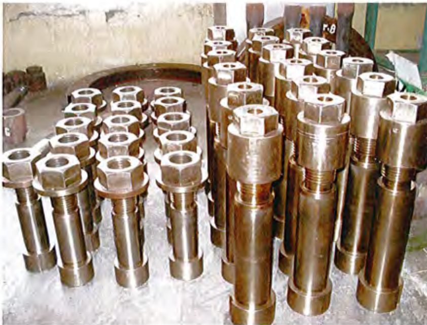
The view of coupling bolt ready for LPT.
