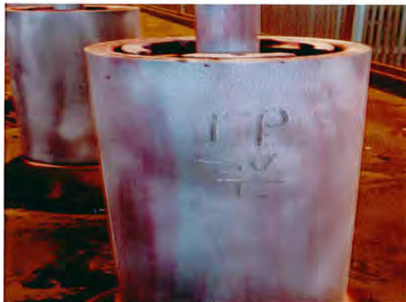
The view of LPT test on IP SV -1
