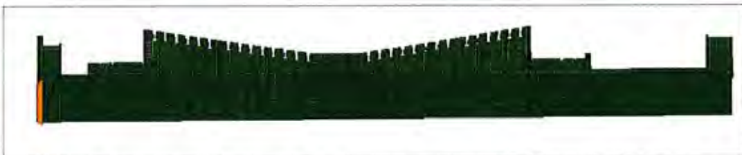
Figure 7:22: Longitudinal Displacement (Y) along Edges of the LP Shaft (Cut Section) is constrained
