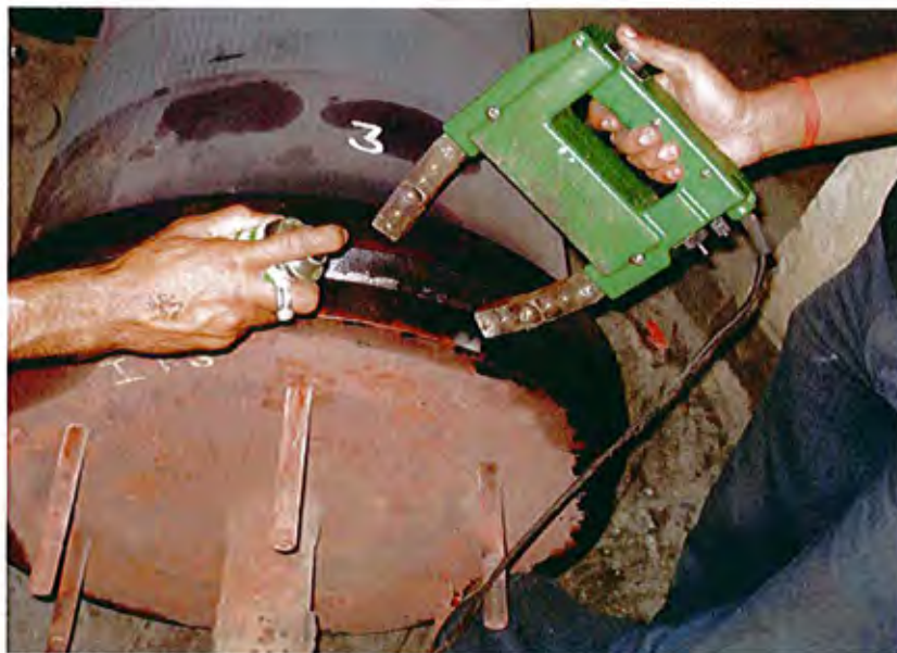
The view of MPI testing on strainer.
