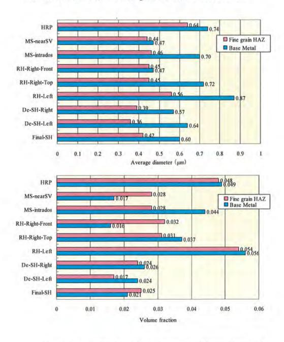
Quantitative evaluation of grain boundary precipitates [extracted Table II -7]
