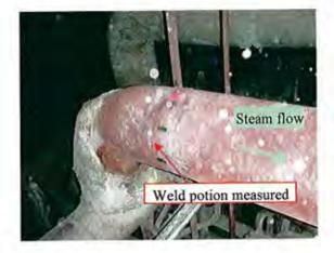
Measurement point of right De-superheater pipe
