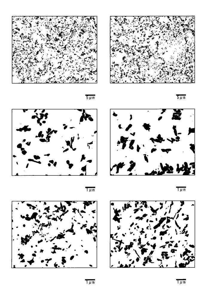
Photo II -7-12 Precipitates by TEM (Transmission electron microscope) observation RH Outlet Header (Circumferential weld at left side: Fine grain HAZ)
