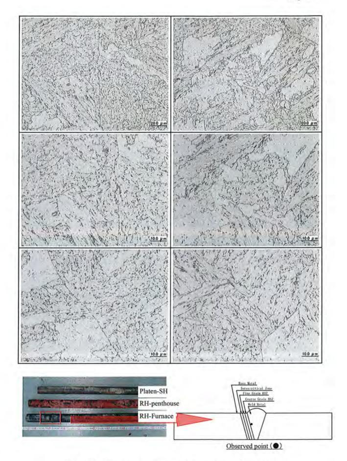
Photo I -52 Microstructure observation at cross section of sample tube [RH-Furnace (Weld Metal) ]
