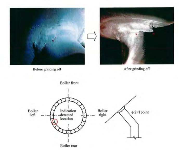
Fig. II-6 The indication pattern detected location
