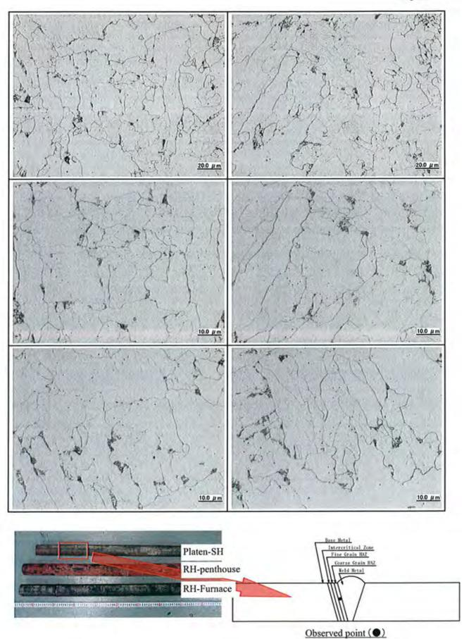
Photo I -29 Microstructure observation at cross section of sample tube [Platen-SH (Coarse Grain HAZ)]
