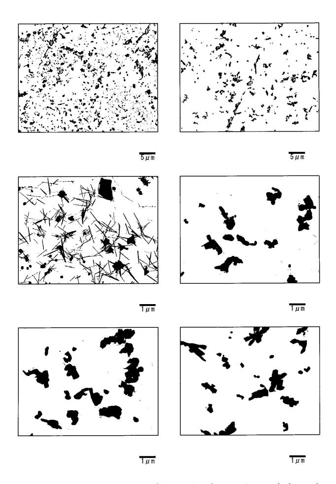
Photo II -11-13 Precipitates by TEM (Transmission electron microscope) observation Main Steam Pipe-Right (Circumferential weld, near the stop valve: Coarse grain HAZ)
