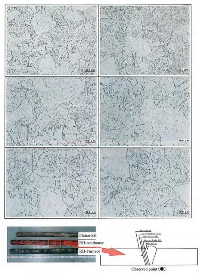
Photo I -37 Microstructure observation at cross section of sample tube [RH-Penthouse (Base Metal)]
