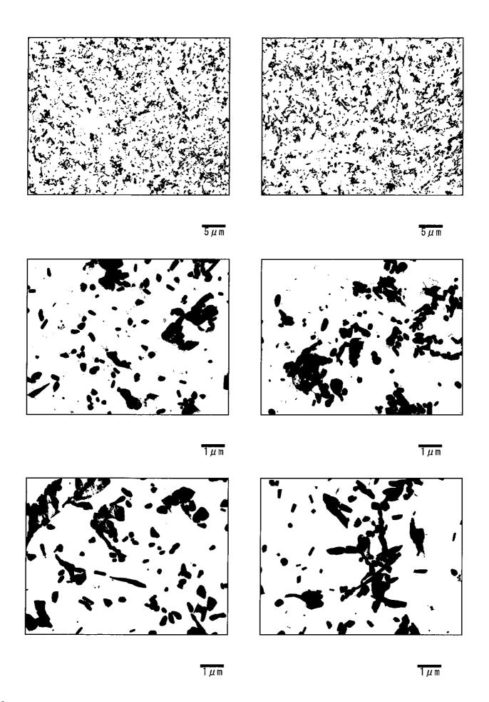
Photo  $\Pi$ -9-12 Precipitates by TEM (Transmission electron microscope) observation RH Outlet Header (Circumferential weld at right side, front : Fine grain HAZ)
