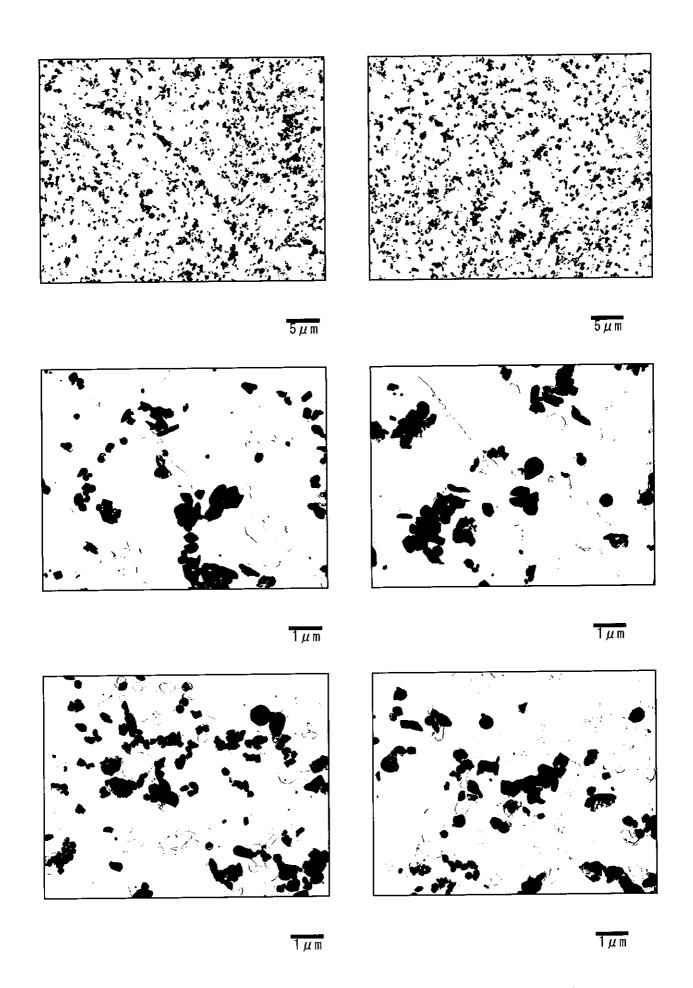
Photo II-12-14 Precipitates by TEM (Transmission electron microscope) observation Hot Reheat Pipe-Right(Circumferential weld: Weld metal)
