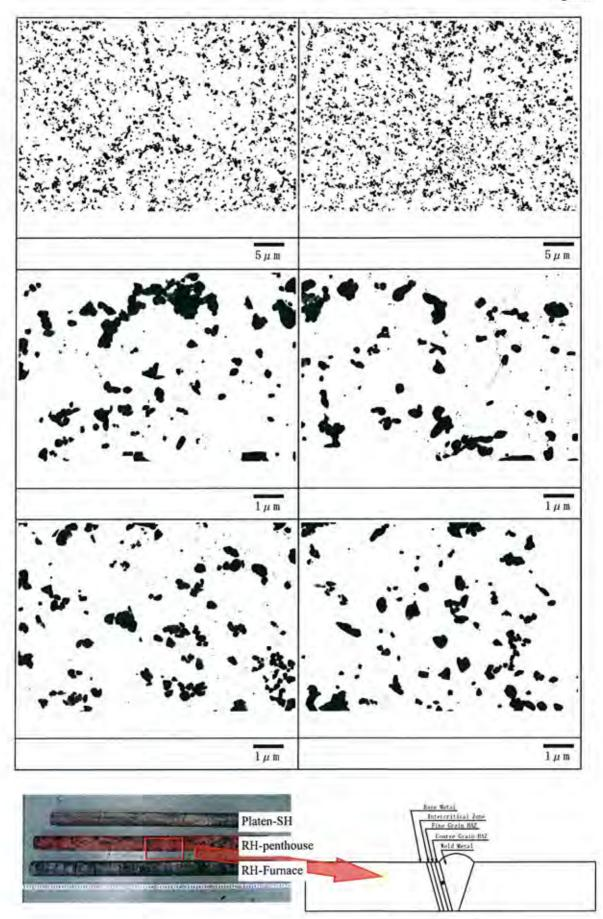
Photo I -46 Precipitates distribution by TEM observation [RH-Penthouse (Coarse Grain HAZ) ]
