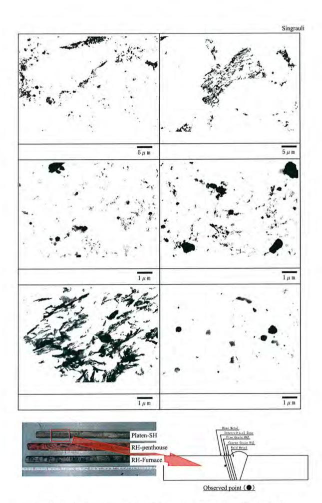
Photo I -33 Precipitates distribution by TEM observation [Platen-SH (Base Metal) ]
