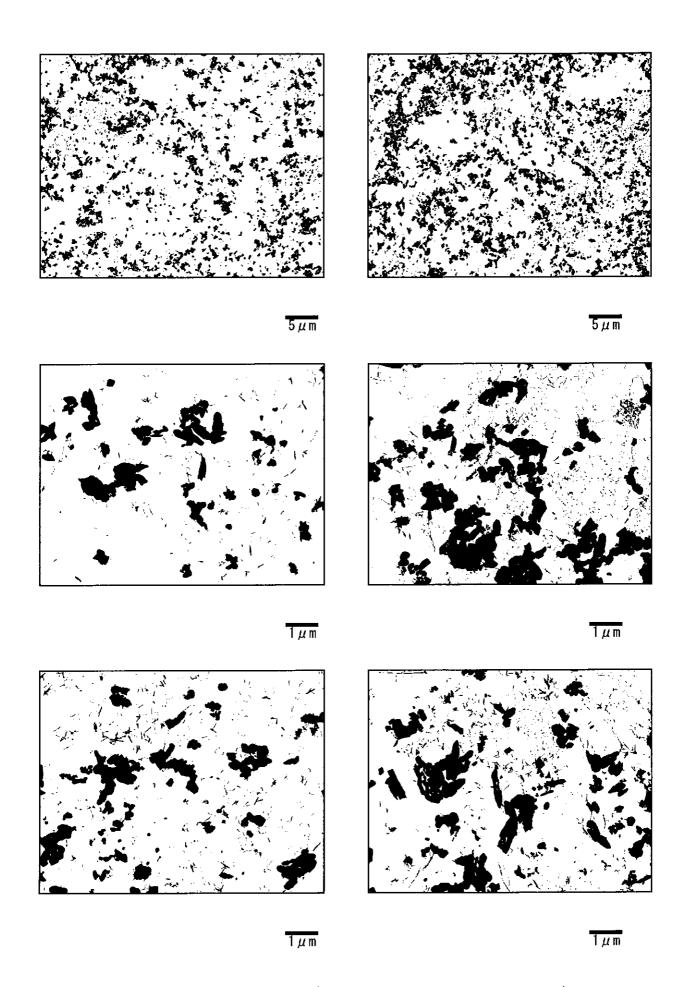
Photo II -5-12 Precipitates by TEM (Transmission electron microscope) observation De-Superheater-Left (Circumferential weld: Fine grain HAZ)
