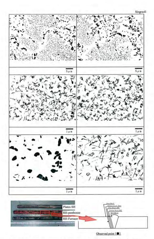
Photo I -44 Precipitates distribution by TEM observation [RH-Penthouse (Base Metal) ]
