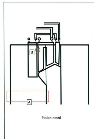
A: Erosion of water wall tube around short soot blowers.
