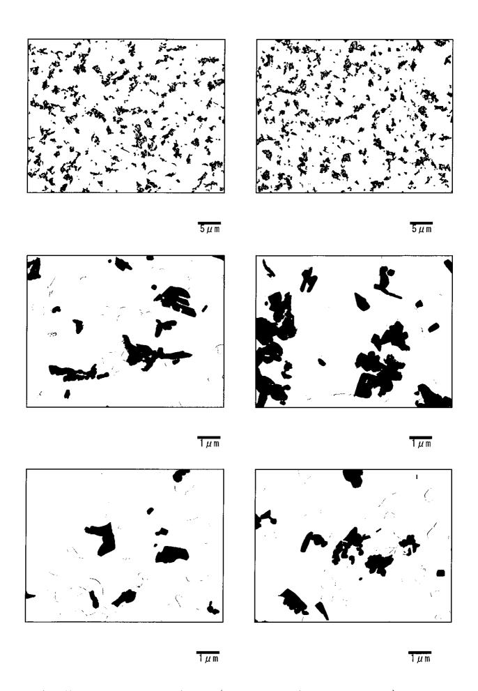
Photo II -11-12 Precipitates by TEM (Transmission electron microscope) observation Main Steam Pipe-Right (Circumferential weld, near the stop valve: Fine grain HAZ)
