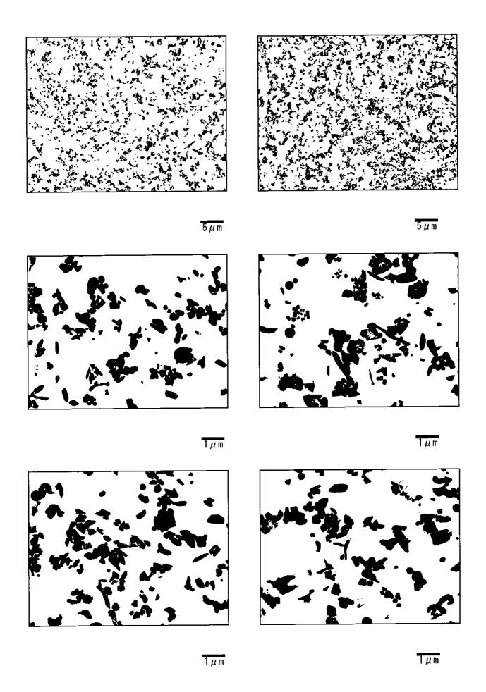
Photo II-10-14 Precipitates by TEM (Transmission electron microscope) observation Main Steam Pipe-Right (Circumferential weld, intrados: Weld metal)
