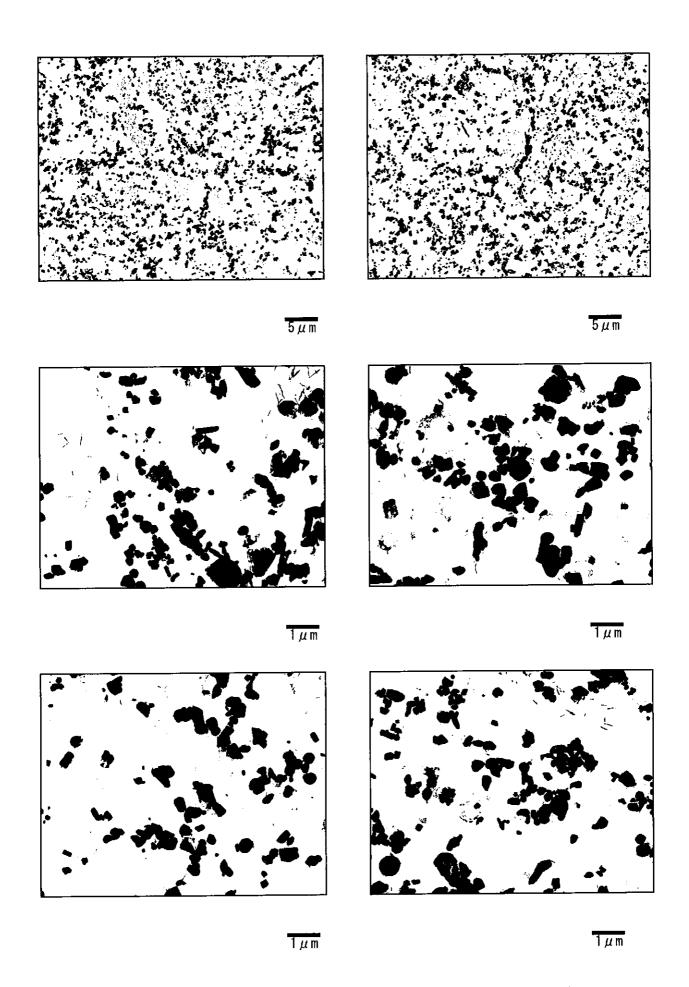
Photo II-12-13 Precipitates by TEM (Transmission electron microscope) observation Hot Reheat Pipe-Right (Circumferential weld: Coarse grain HAZ)
