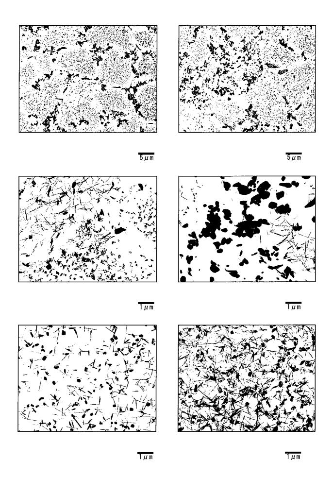
Photo  $\Pi$ -10-11 Precipitates by TEM (Transmission electron microscope) observation Main Steam Pipe-Right (Circumferential weld, intrados: Base metal)
