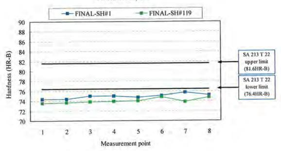
Fig II -25 Hardness measurement results
