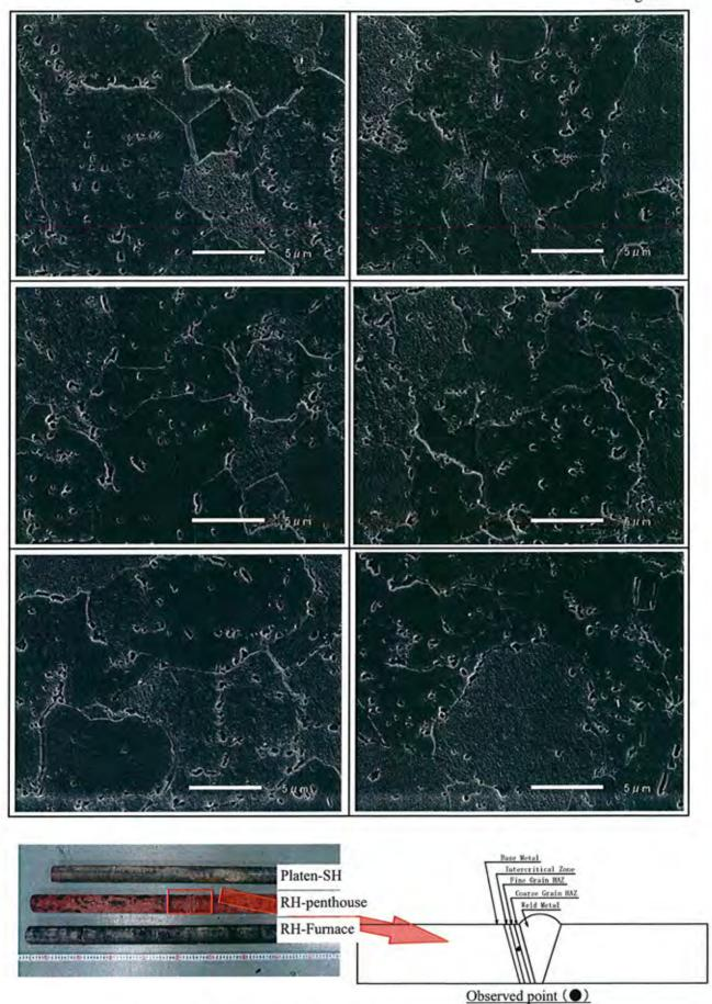
Photo I -43 Precipitates along grain boundary by SEM observation [RH-Penthouse (Fine Grain HAZ)]
