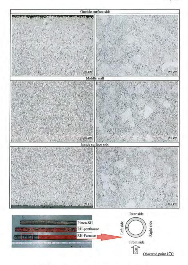
Photo I -25 Microstructure observation at cross section of sample tube [RH-Furnace (left side, Base Metal)]
