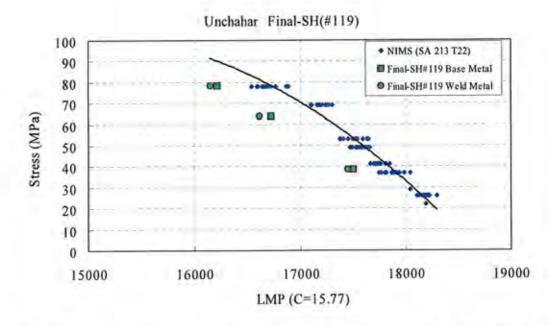
Fig II-27 The comparison of the test results and the creep rupture data of virgin materials by NIMS (National Institute for Materials science).
