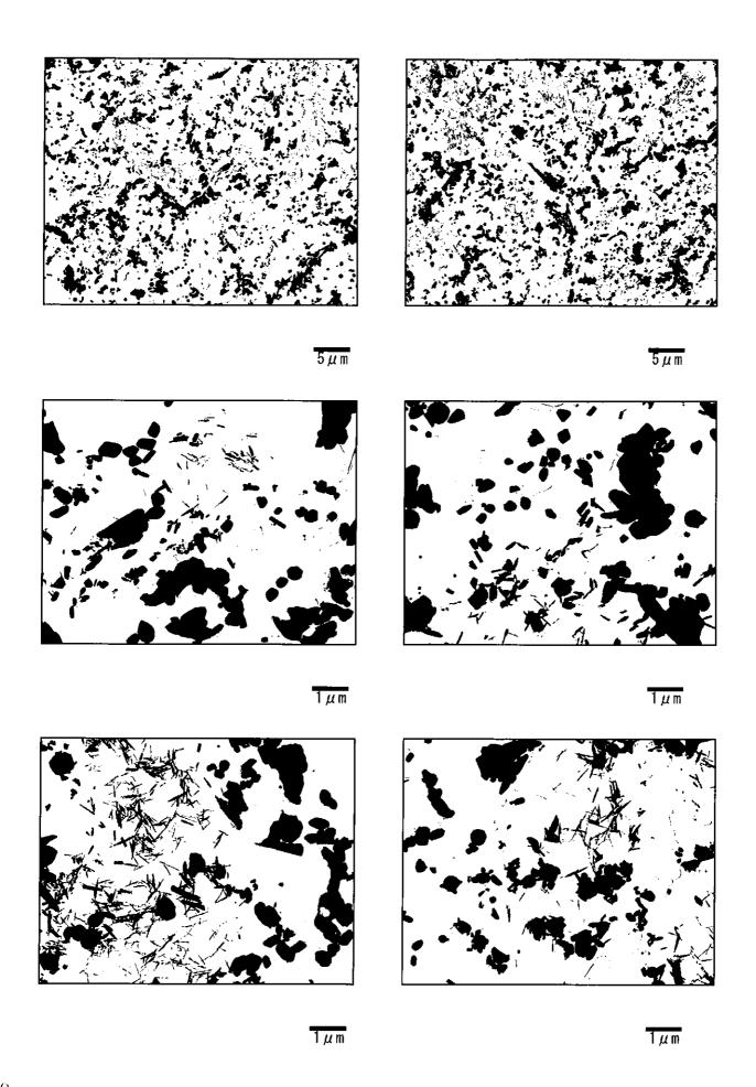
Photo II-8-13 Precipitates by TEM (Transmission electron microscope) observation RH Outlet Header (Circumferential weld at right side, top : Coarse grain HAZ)
