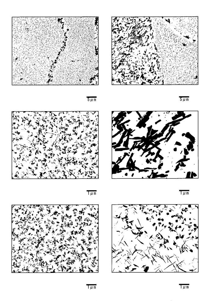
Photo II -7-11 Precipitates by TEM (Transmission electron microscope) observation RH Outlet Header (Circumferential weld at left side: Base metal)
