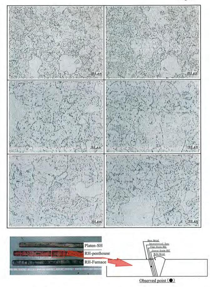
Photo I -38 Microstructure observation at cross section of sample tube [RH-Penthouse (Intercritical Zone)]
