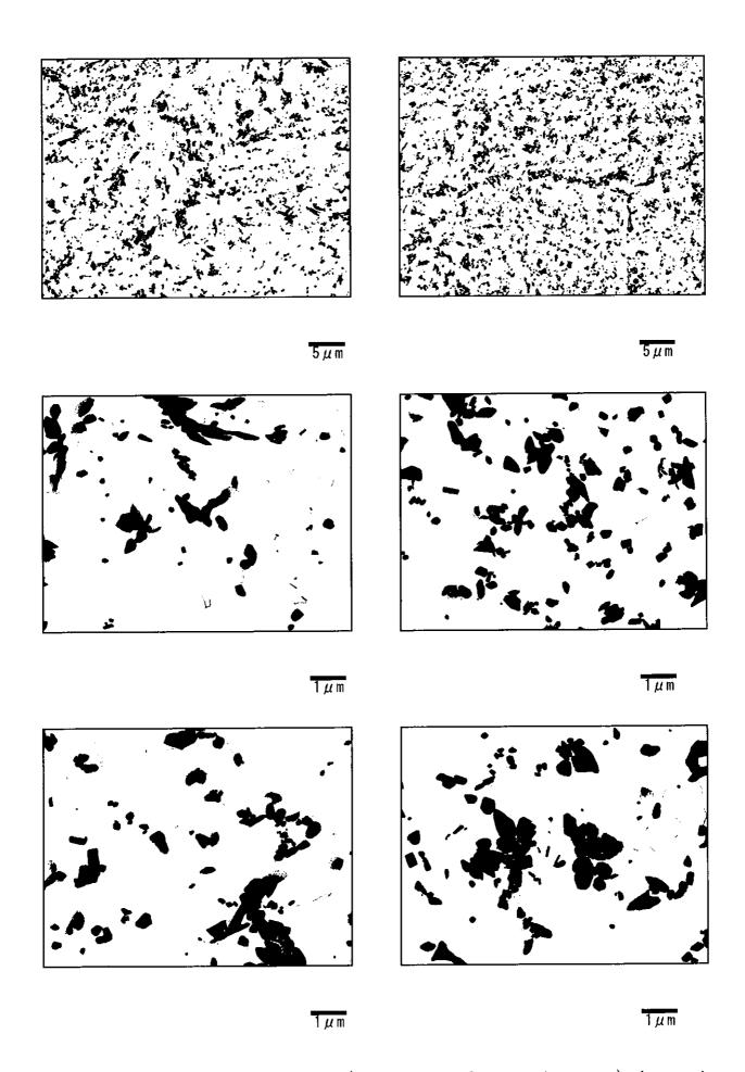
Photo II-10-13 Precipitates by TEM (Transmission electron microscope) observation Main Steam Pipe-Right (Circumferential weld, intrados: Coarse grain HAZ)
