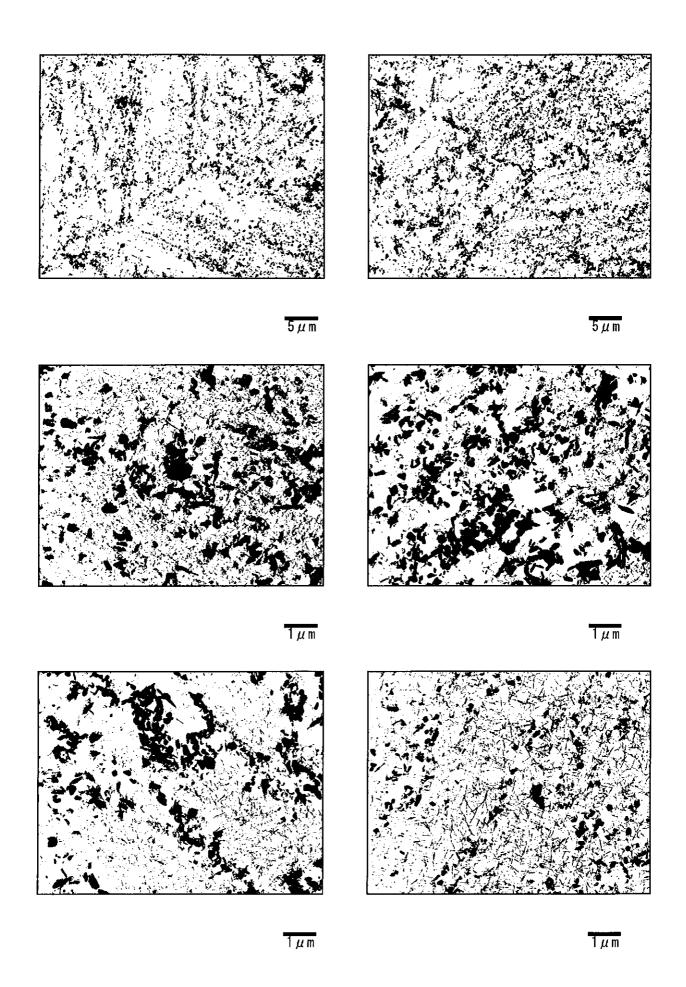
Photo II -6-13 Precipitates by TEM (Transmission electron microscope) observation De-Superheater-Right (Circumferential weld: Coarse grain HAZ)
