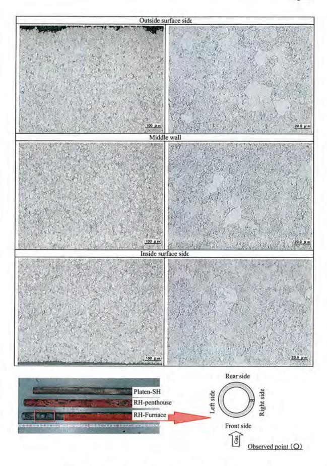
Photo I -24 Microstructure observation at cross section of sample tube [RH-Furnace (right side, Base Metal)]
