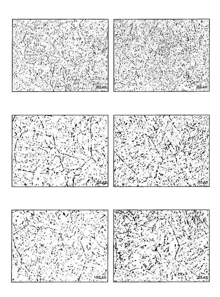
Photo II -7-4 Microstructure observation RH Outlet Header (Circumferential weld at left side : Coarse grain HAZ )
