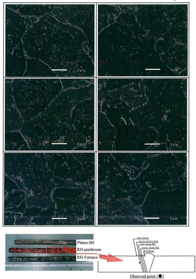
Photo I -42 Precipitates along grain boundary by SEM observation [RH-Penthouse (Base Metal)]
