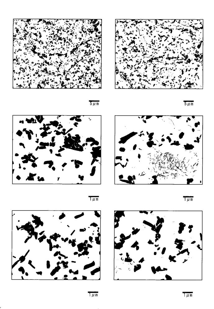
Photo II -4-13 Precipitates by TEM (Transmission electron microscope) observation Final SH Outlet Header (Circumferential weld at right side: Coarse grain HAZ)
