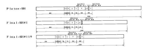
1: Outer surface appearance 2: Internal surface appearance 3: Tube dimension • Hardness 4: Metallography 5: Scale thickness, EPMA analysis, 6: RLA by microstructural comparison method 7: Creep rupture test
