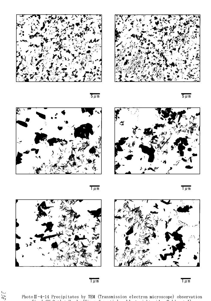
Photo II -4-14 Precipitates by TEM (Transmission electron microscope) observation Final SH Outlet Header(Circumferential weld at right side: Weld metal)
