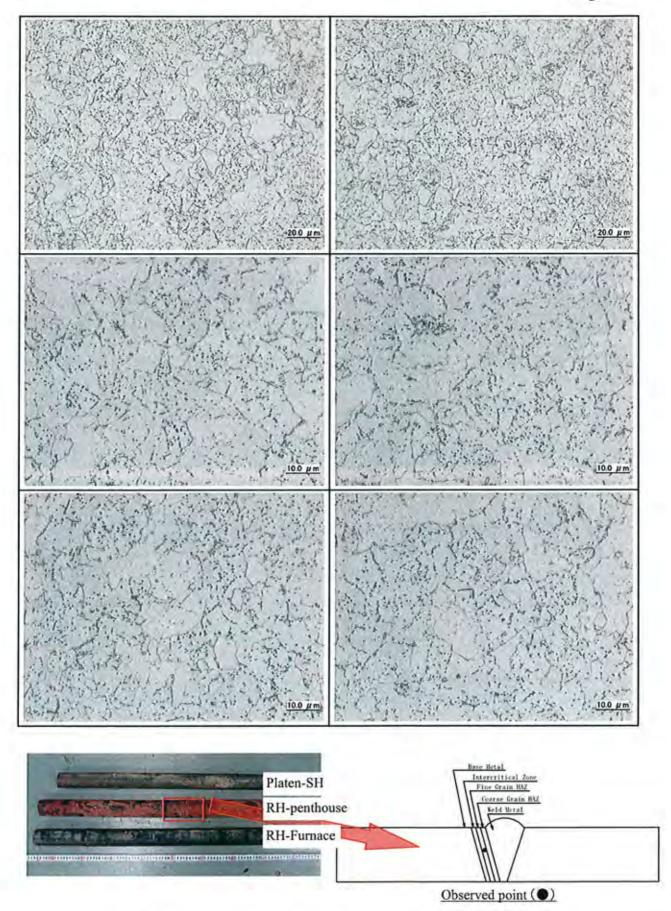
Photo I -39 Microstructure observation at cross section of sample tube [RH-Penthouse (Fine Grain HAZ)]
