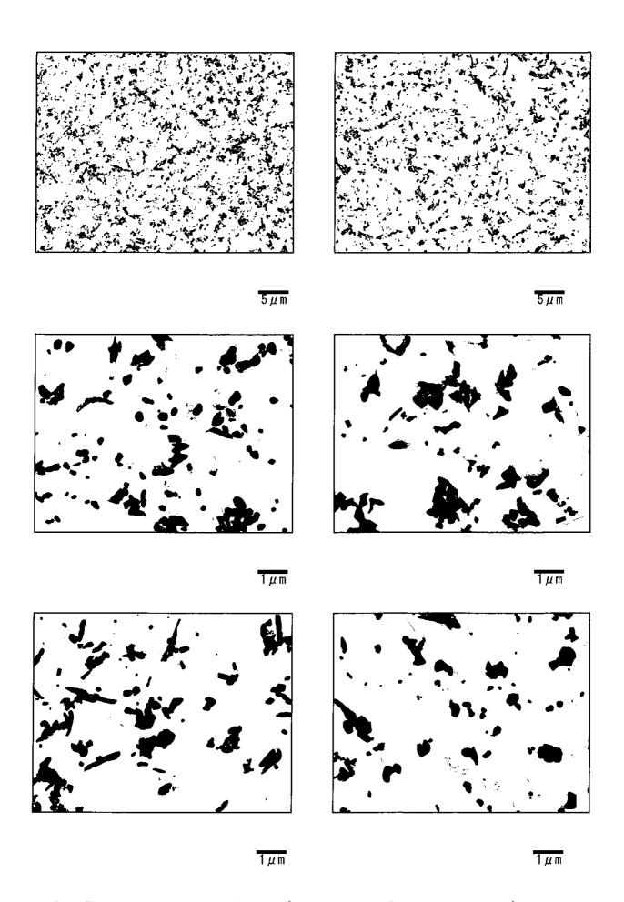
Photo II-10-12 Precipitates by TEM (Transmission electron microscope) observation Main Steam Pipe-Right (Circumferential weld, intrados: Fine grain HAZ)
