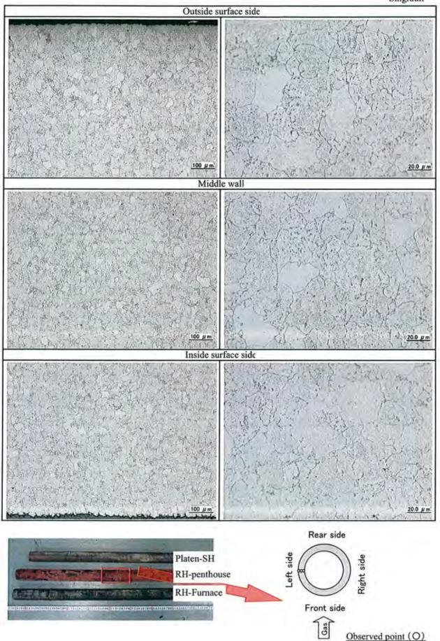
Photo I -23 Microstructure observation at cross section of sample tube [RH-Penthouse (right side, Base Metal)]
