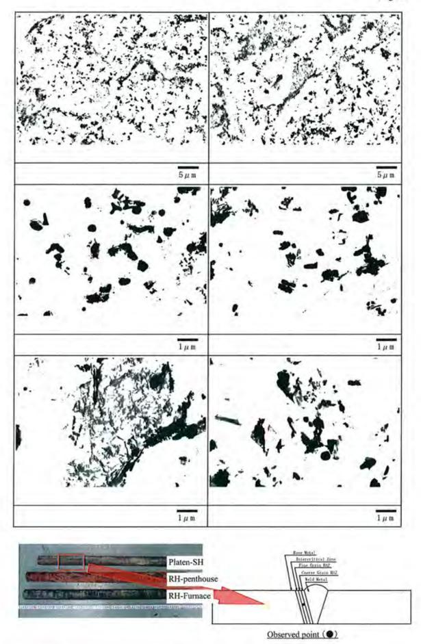
Photo I -34 Precipitates distribution by TEM observation [Platen-SH (Fine Grain HAZ) ]
