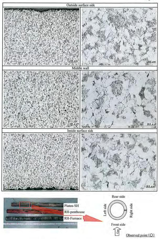
Photo I -20 Microstructure observation at cross section of sample tub-[Platen-SH (right side, Base Metal)]
