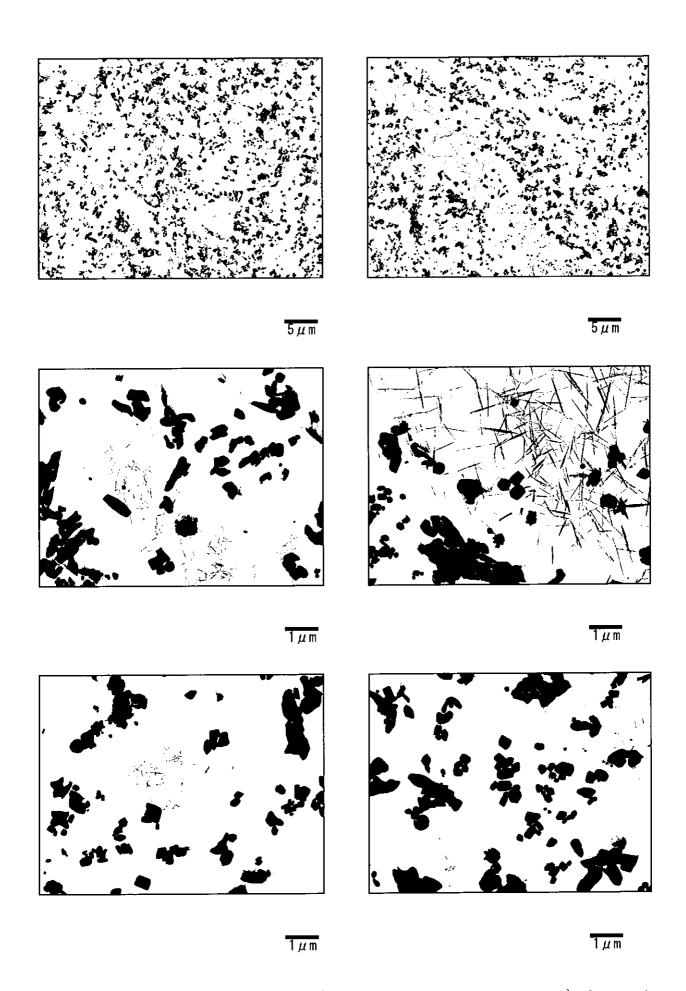
Photo II-11-14 Precipitates by TEM (Transmission electron microscope) observation Main Steam Pipe-Right (Circumferential weld, near the stop valve: Weld metal)
