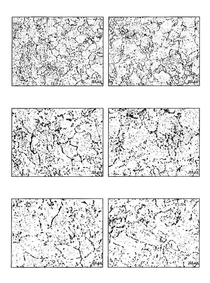
$Photo\,\Pi\,\hbox{--}12\hbox{--}2\quad Microstructure\ observation}\\ Hot\ Reheat\ Pipe-Right\ (Circumferential\ weld\ : Intercritical\ zone\ )$
