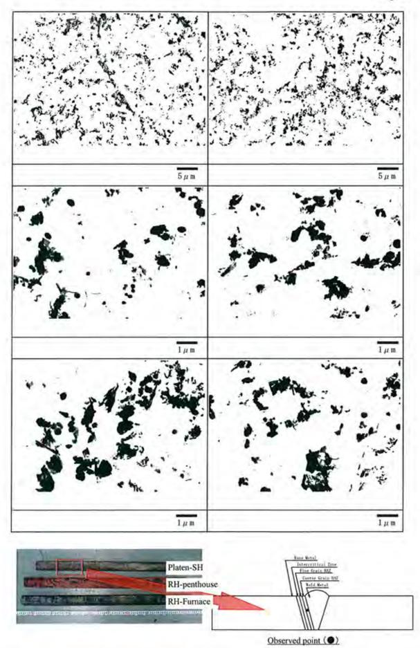
Photo I -35 Precipitates distribution by TEM observation [Platen-SH (Coarse Grain HAZ) ]
