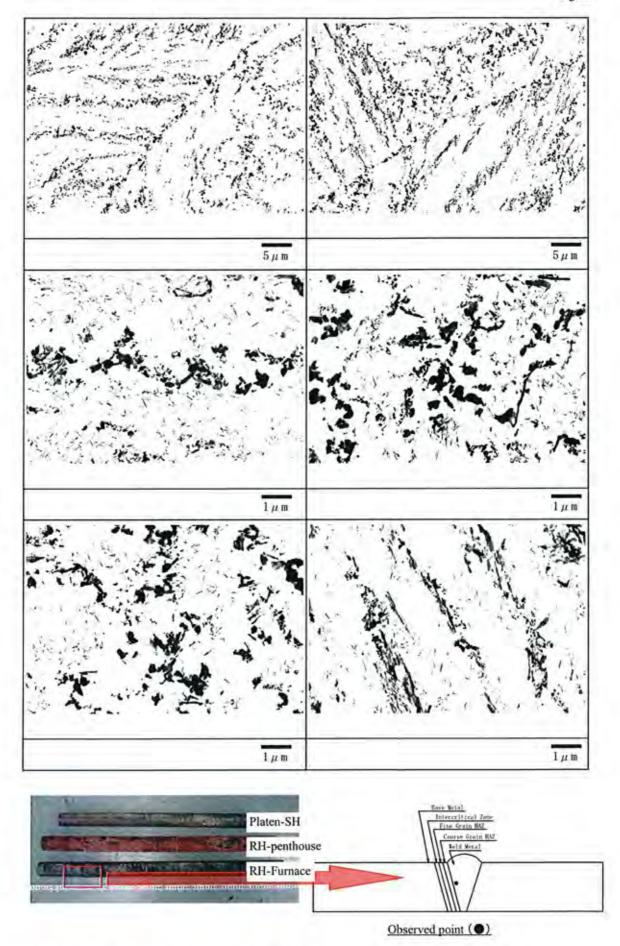
Photo I -58 Precipitates distribution by TEM observation [RH-Furnace (Weld Metal) ]
