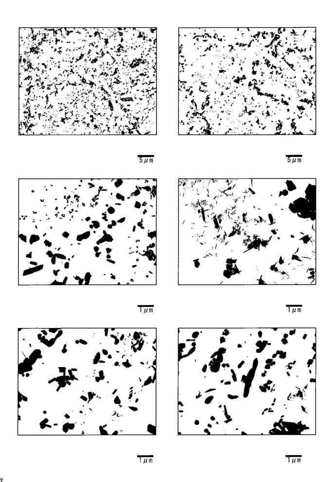
Photo II -9-13 Precipitates by TEM (Transmission electron microscope) observation RH Outlet Header(Circumferential weld at right side, front : Coarse grain HAZ)
