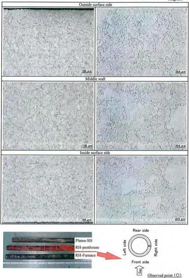
Photo I -22 Microstructure observation at cross section of sample tube [RH-Penthouse (right side, Base Metal)]
