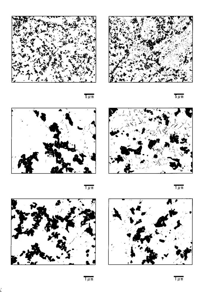
Photo II -5-13 Precipitates by TEM (Transmission electron microscope) observation De-Superheater-Left(Circumferential weld: Coarse grain HAZ)
