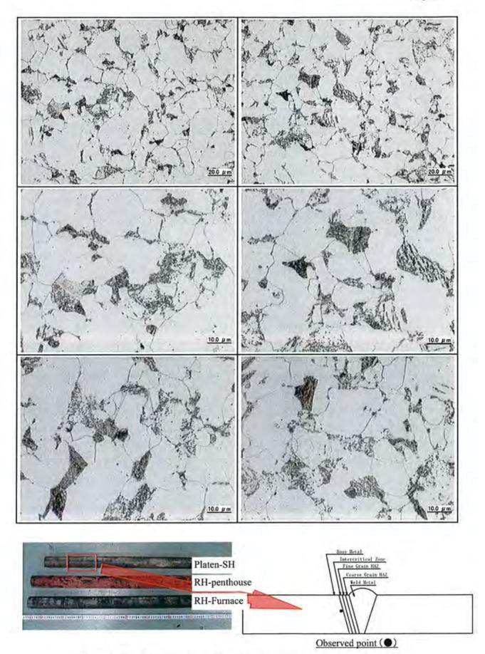
Photo I -26 Microstructure observation at cross section of sample tube [Platen-SH (Base Metal)]
