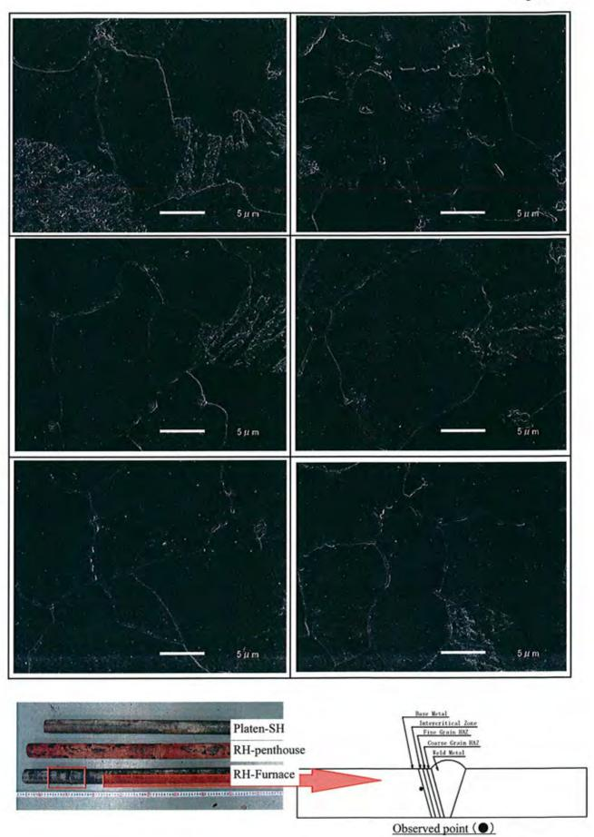
Photo I -53 Precipitates along grain boundary by SEM observation [RH-Furnace (Base Metal)]
