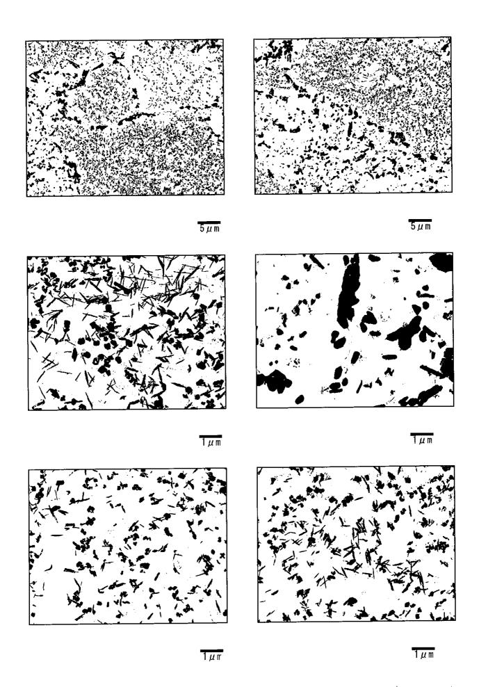
Photo II-12-11 Precipitates by TEM (Transmission electron microscope) observation Hot Reheat Pipe-Right(Circumferential weld: Base metal)
