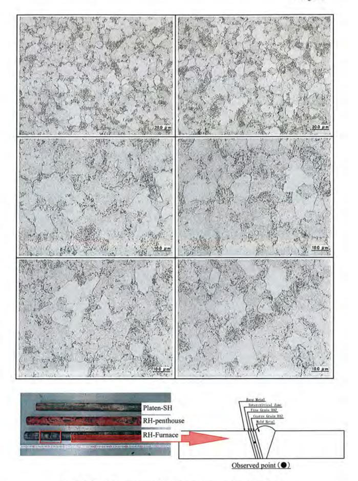
Photo I -50 Microstructure observation at cross section of sample tube [RH-Furnace (Fine Grain HAZ)]
