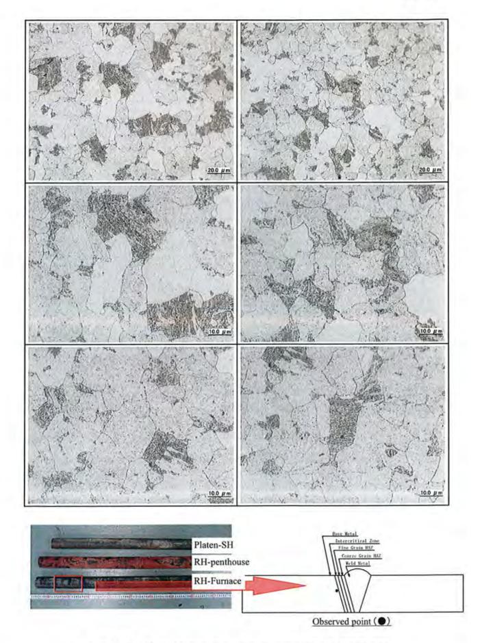
Photo I -48 Microstructure observation at cross section of sample tube [RH-Furnace (Base Metal)]
