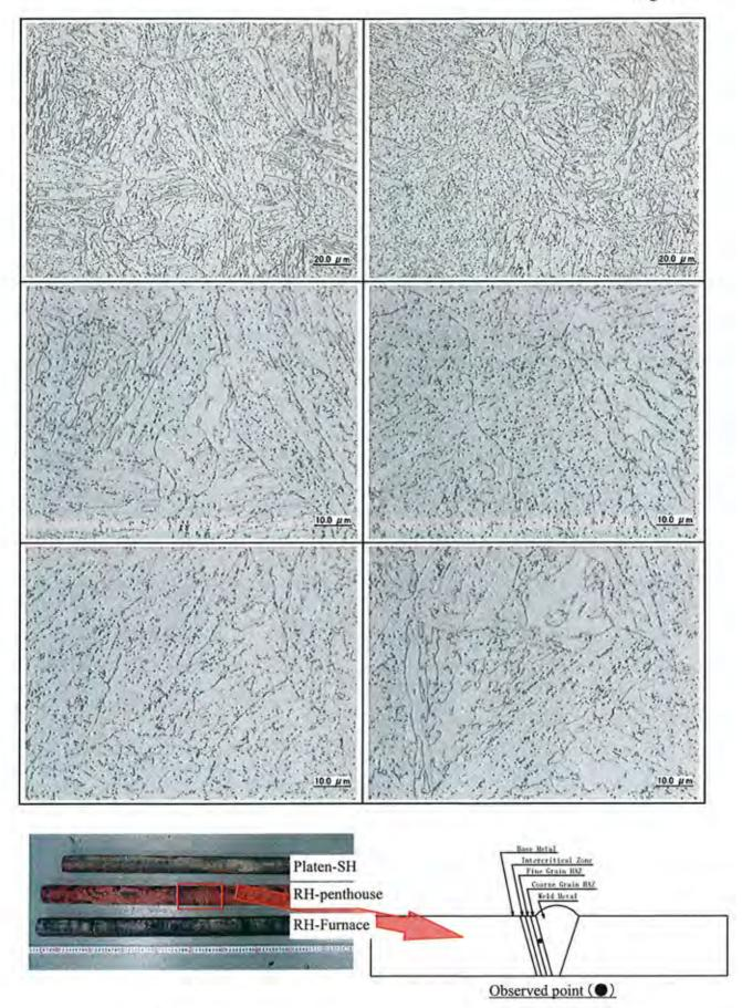
Photo I -40 Microstructure observation at cross section of sample tube [RH-Penthouse (Coarse Grain HAZ)]
