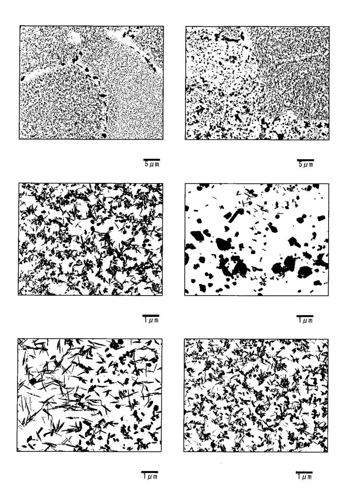
Photo II -4-11 Precipitates by TEM (Transmission electron microscope) observation Final SH Outlet Header(Circumferential weld at right side: Base metal)
