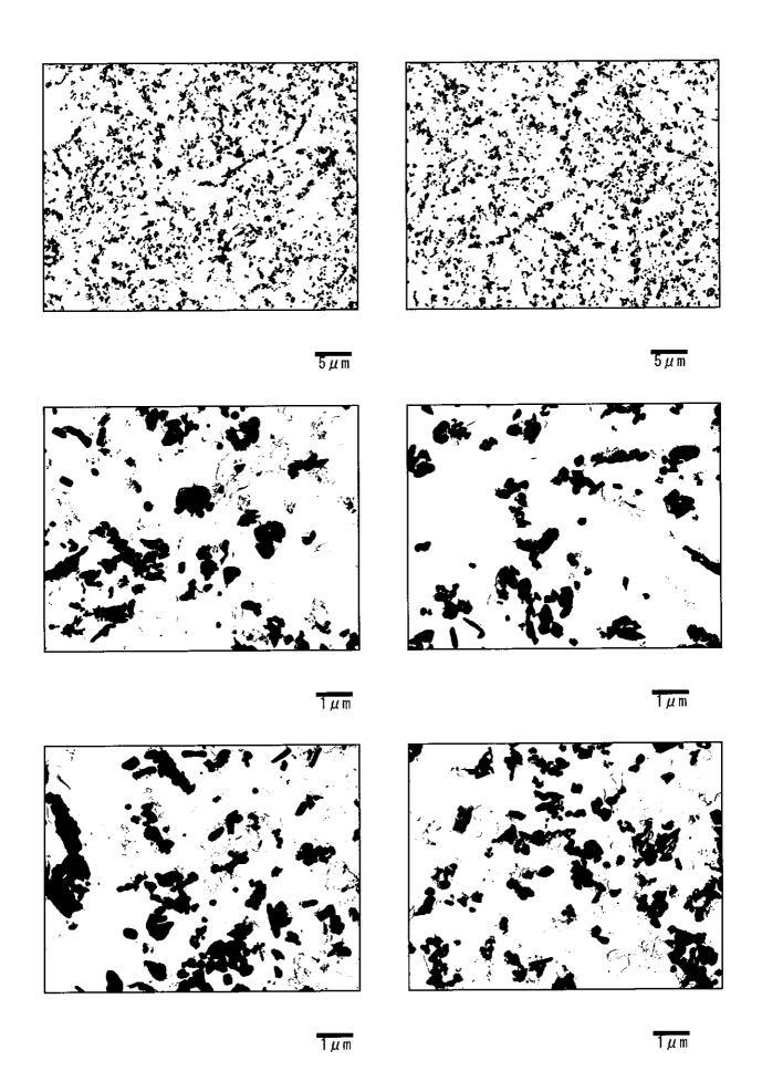
Photo II-12-12 Precipitates by TEM (Transmission electron microscope) observation Hot Reheat Pipe-Right(Circumferential weld: Fine grain HAZ)
