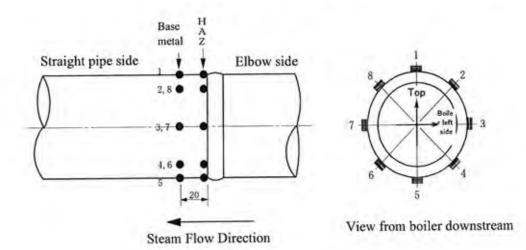
Table II -22 (Unchahar) Re-Heater Outlet Header Outside Diameter Measurement Results
