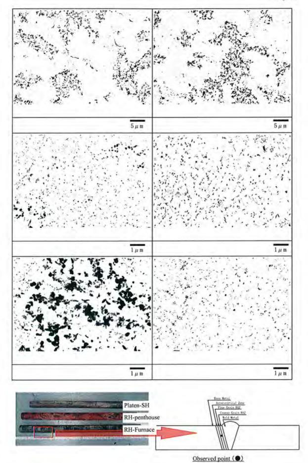
Photo I -56 Precipitates distribution by TEM observation [RH-Furnace (Fine Grain HAZ) ]
