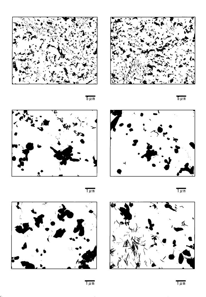
Photo II-8-14 Precipitates by TEM (Transmission electron microscope) observation RH Outlet Header (Circumferential weld at right side, top: Weld metal)
