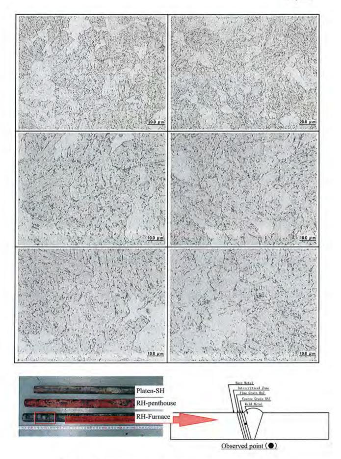
Photo I -51 Microstructure observation at cross section of sample tube [RH-Furnace (Coarse Grain HAZ)]
