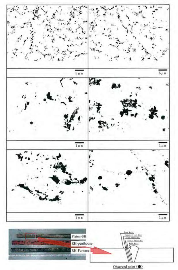
Photo I -36 Precipitates distribution by TEM observation [Platen-SH (Weld Metal) ]
