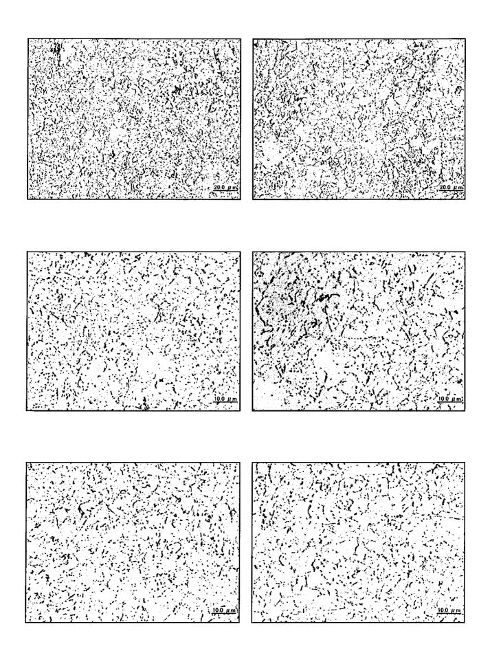
$\label{lem:photoII-9-3} Photo II-9-3 \quad \mbox{Microstructure observation} \\ \mbox{RH Outlet Header (Circumferential weld at right side, front : Fine grain HAZ )}$
