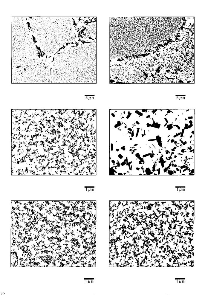
Photo II-8-11 Precipitates by TEM (Transmission electron microscope) observation RH Outlet Header (Circumferential weld at right side, top: Base metal)
