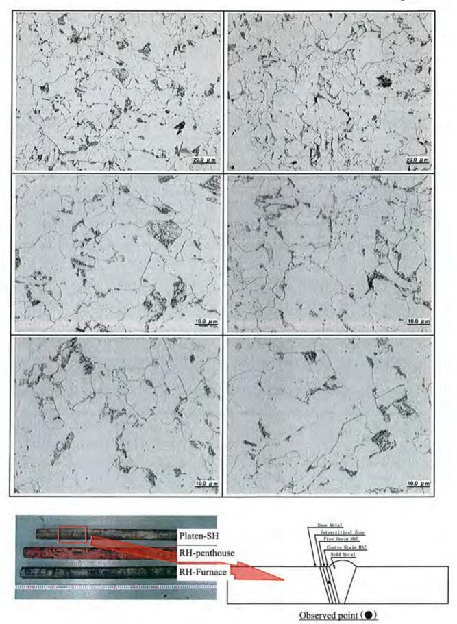
Photo I -28 Microstructure observation at cross section of sample tube [Platen-SH (Fine Grain HAZ)]
