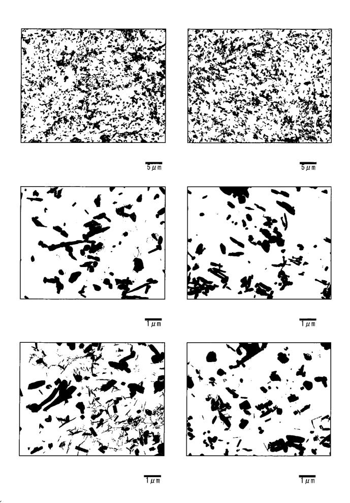
Photo II -4-12 Precipitates by TEM (Transmission electron microscope) observation Final SH Outlet Header(Circumferential weld at right side: Fine grain HAZ)
