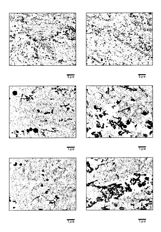
Photo II -6-14 Precipitates by TEM (Transmission electron microscope) observation De-Superheater-Right (Circumferential weld: Weld metal)
