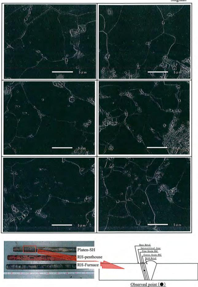
Photo I -32 Precipitates along grain boundary by SEM observatior [Platen-SH (Fine Grain HAZ) ]
