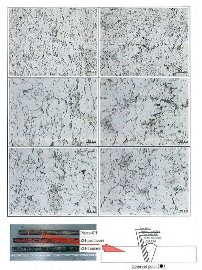
Photo I -30 Microstructure observation at cross section of sample tube [Platen-SH (Weld Metal)]
