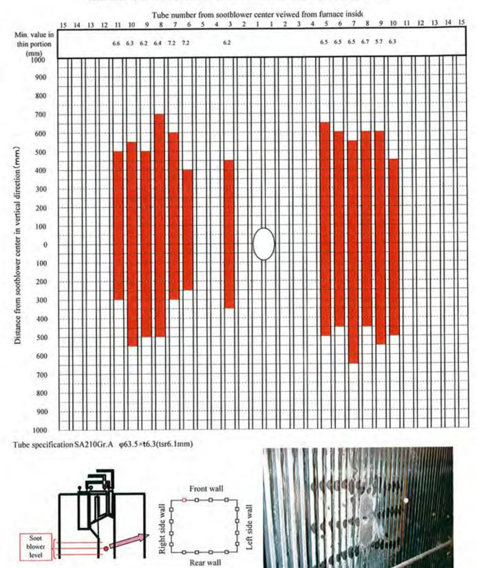
Table II-14 (Unchahar) WATER WALL Rear wall Thickness Measurement Results
