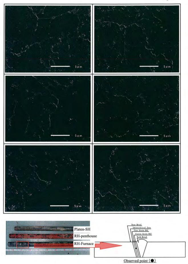
Photo I -54 Precipitates along grain boundary by SEM observation [RH-Furnace (Fine Grain HAZ) ]
