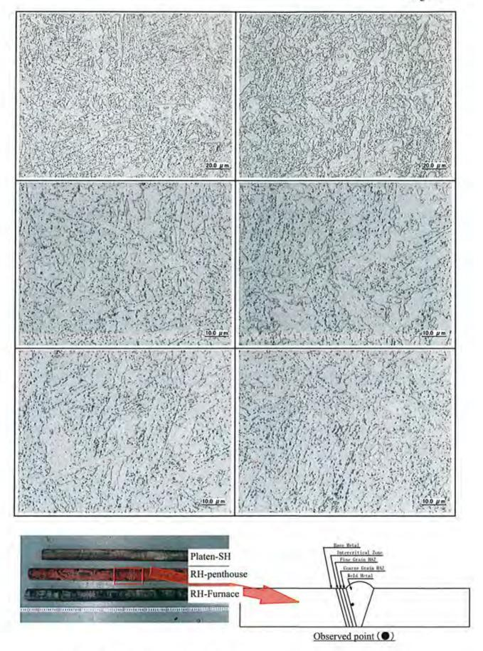
Photo I -41 Microstructure observation at cross section of sample tube [RH-Penthouse (Weld Metal)]
