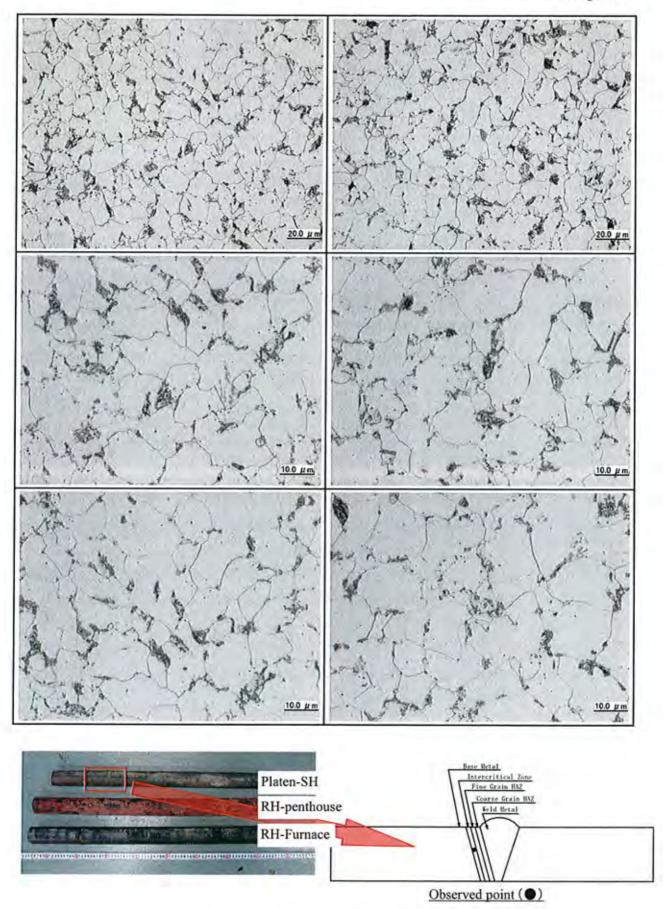
Photo I -27 Microstructure observation at cross section of sample tube [Platen-SH (Intercritical Zone)]
