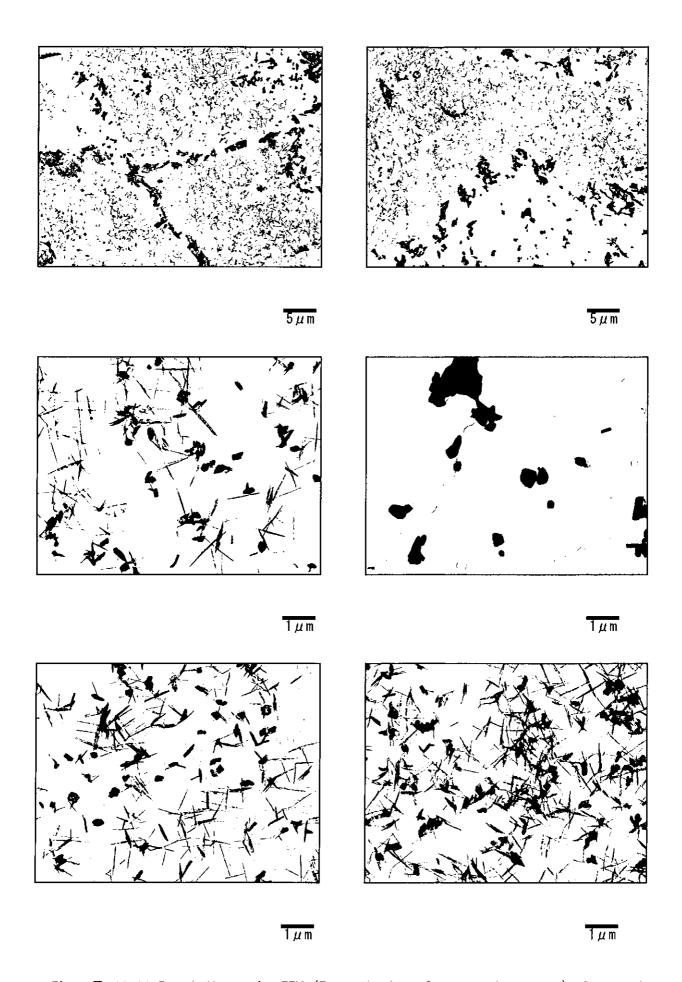
Photo II-11-11 Precipitates by TEM (Transmission electron microscope) observation Main Steam Pipe-Right (Circumferential weld, near the stop valve: Base metal)
