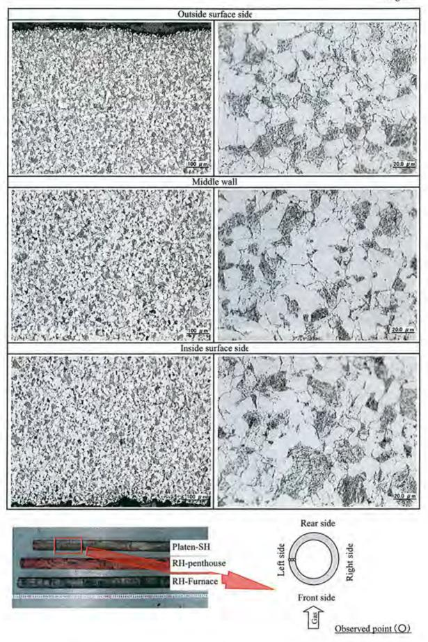
Photo I -21 Microstructure observation at cross section of sample tub [Platen-SH (left side, Base Metal)]
