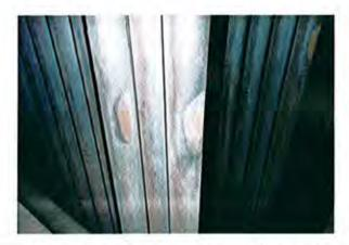
Erosion of Platen SH tube at the highest level of soot blower [extracted from Table II-18]
