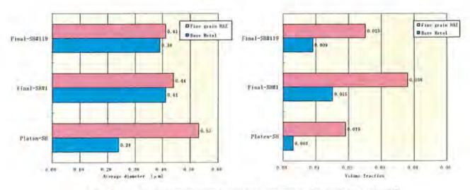
Quantitative evaluation of grain boundary precipitates [extracted Table II -41]
