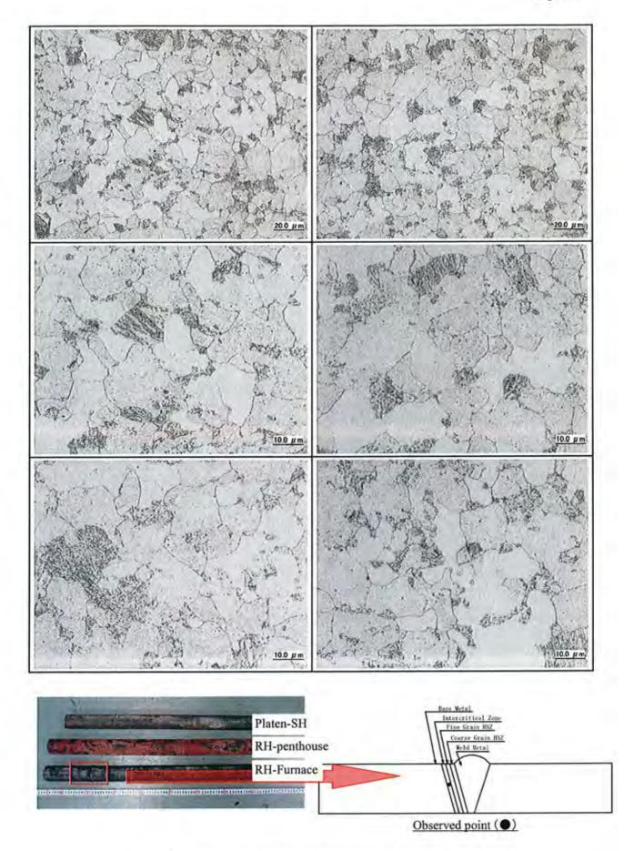
Photo I -49 Microstructure observation at cross section of sample tube [RH-Furnace (Intercritical Zone)]
