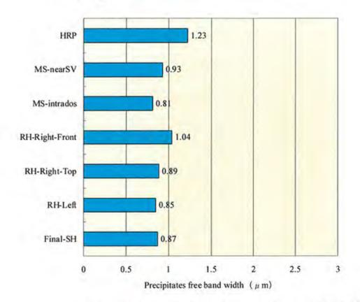
Precipitates free band width along grain boundary [extracted Table II-8]
