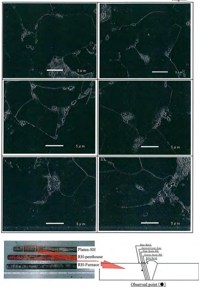
Photo I -31 Precipitates along grain boundary by SEM observation [Platen-SH (Base Metal)]
