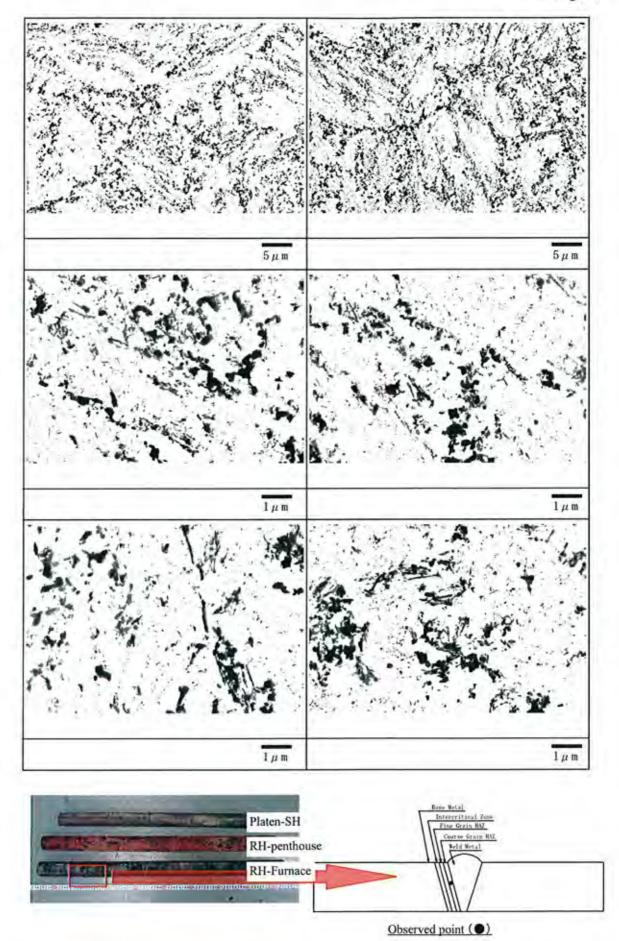
Photo 1 -57 Precipitates distribution by TEM observation [RH-Furnace (Coarse Grain HAZ) ]
