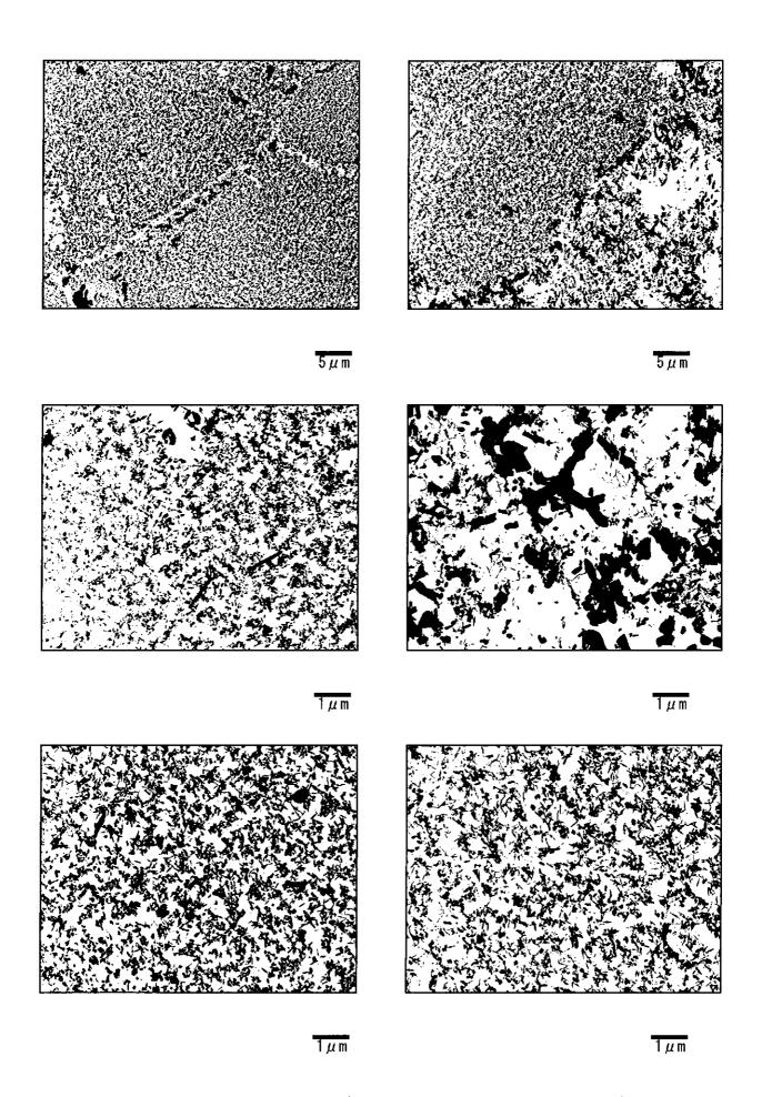
Photo II -5-11 Precipitates by TEM (Transmission electron microscope) observation De-Superheater-Left (Circumferential weld: Base metal)
