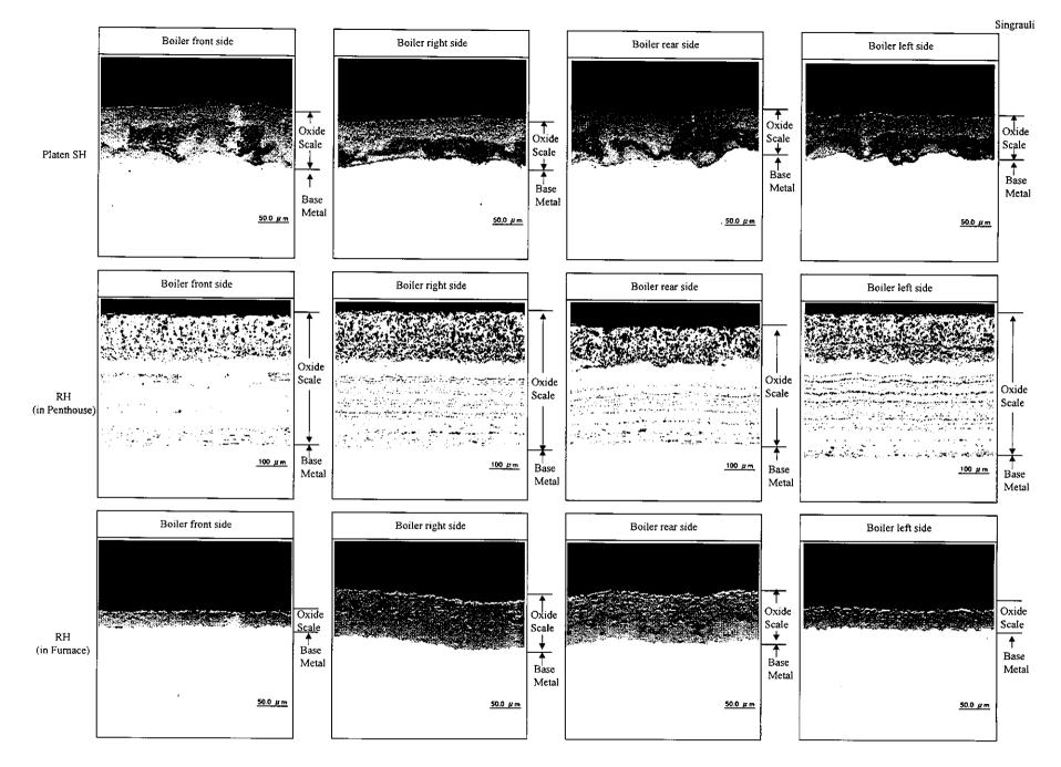
Photo I -19 Cross sectional observation of sample tube inside surface
