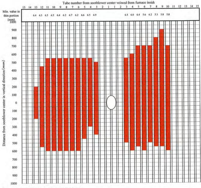
Tube specification SA210Gr.A \( \phi 63.5 \times t6.3 (tsr6.1mm) \)
