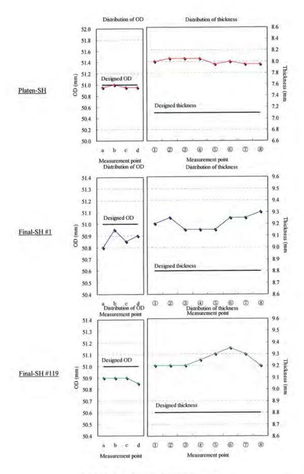
Fig II -12 Tube dimension measurement results
