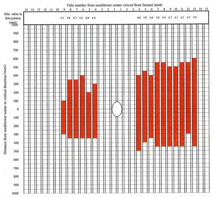
Tube specification SA210Gr.A φ63.5×t6.3(tsr6.1mm)
