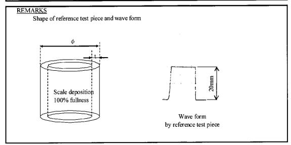
SUS scale deposition inspection was carried out at outer most tube bottom bend and horizontal portion of Platen-SH as shown in Fig. II -2.
