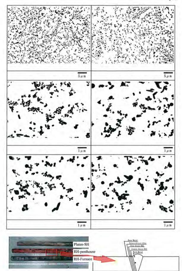
Photo I -47 Precipitates distribution by TEM observation (RH-Penthouse (Weld Metal) )
