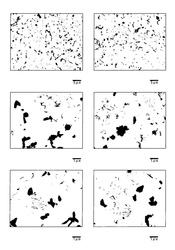
Photo II-7-14 Precipitates by TEM (Transmission electron microscope) observation RH Outlet Header (Circumferential weld at left side: Weld metal)
