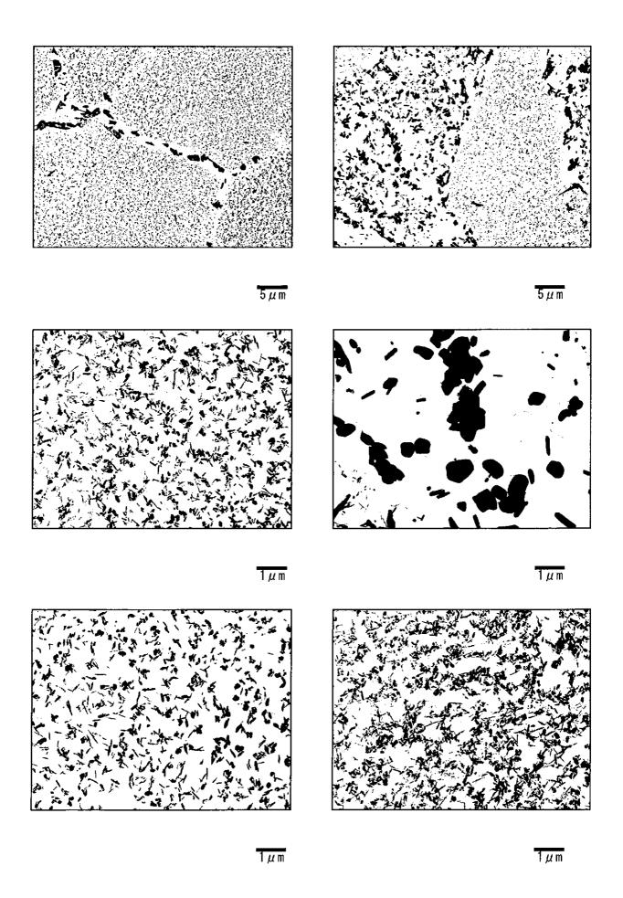
Photo II -9-11 Precipitates by TEM (Transmission electron microscope) observation RH Outlet Header (Circumferential weld at right side, front : Base metal)
