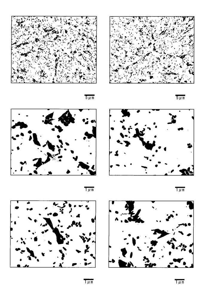
Photo  $\Pi$  -7-13 Precipitates by TEM (Transmission electron microscope) observation RH Outlet Header(Circumferential weld at left side: Coarse grain HAZ)
