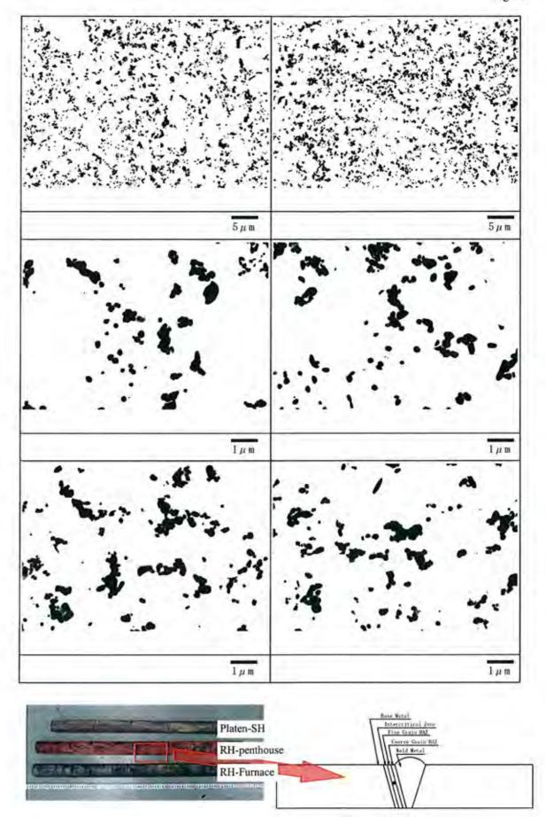
Photo I -45 Precipitates distribution by TEM observation [RH-Penthouse (Fine Grain HAZ) ]
