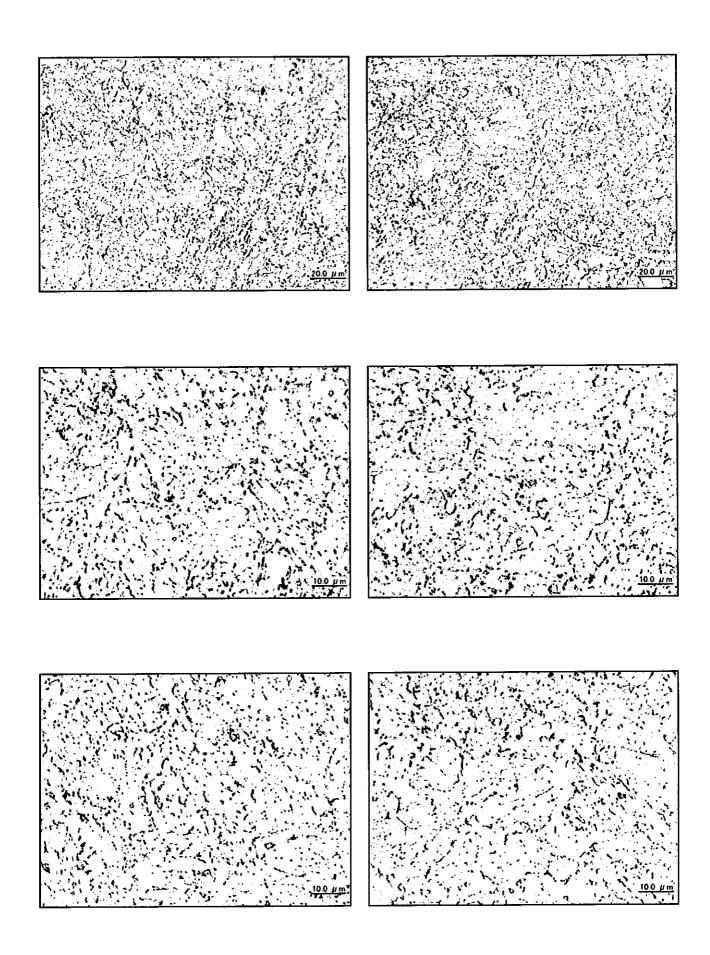
$Photo \ \Pi-11-5 \quad Microstructure \ observation \\ Main \ Steam \ Pipe-Right \ (Circumferential \ weld, near \ the \ stop \ valve \ : Weld \ metal \ )$
