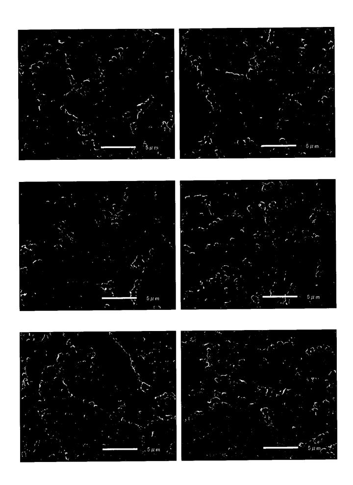
Photo II -12-10 Precipitates along grain boundary by SEM observation Hot Reheat Pipe-Right (Circumferential weld: Fine grain HAZ)
