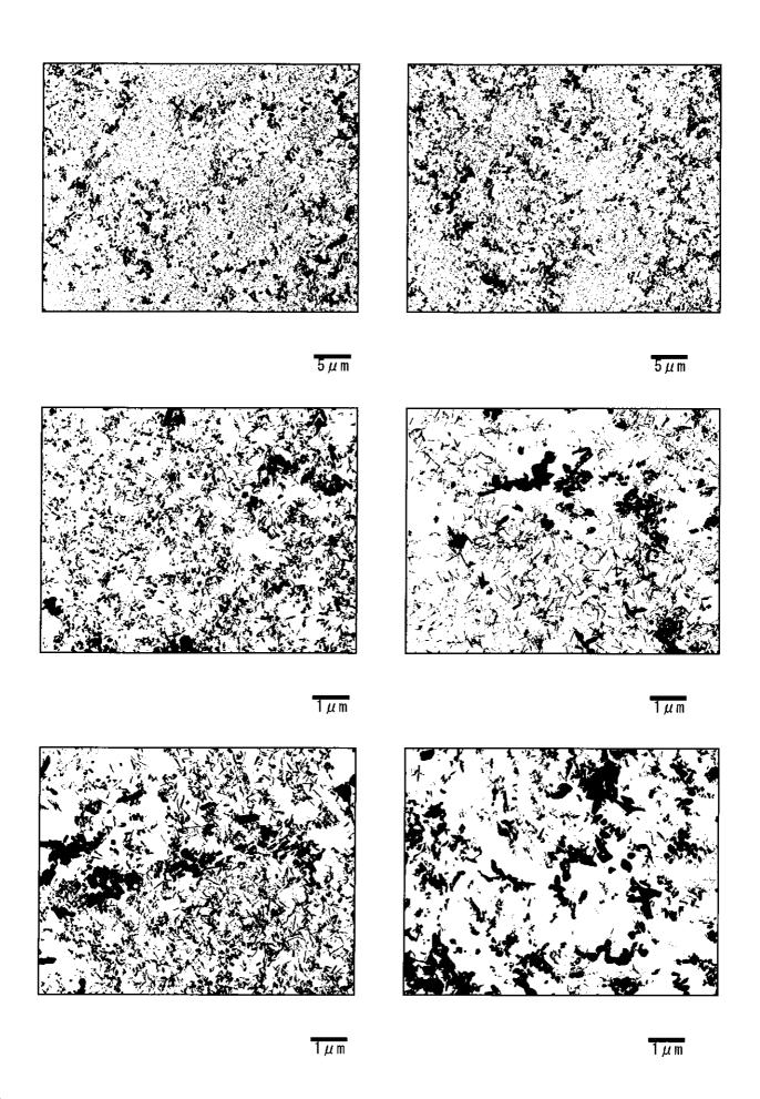
Photo II -6-12 Precipitates by TEM (Transmission electron microscope) observation De-Superheater-Right (Circumferential weld: Fine grain HAZ)
