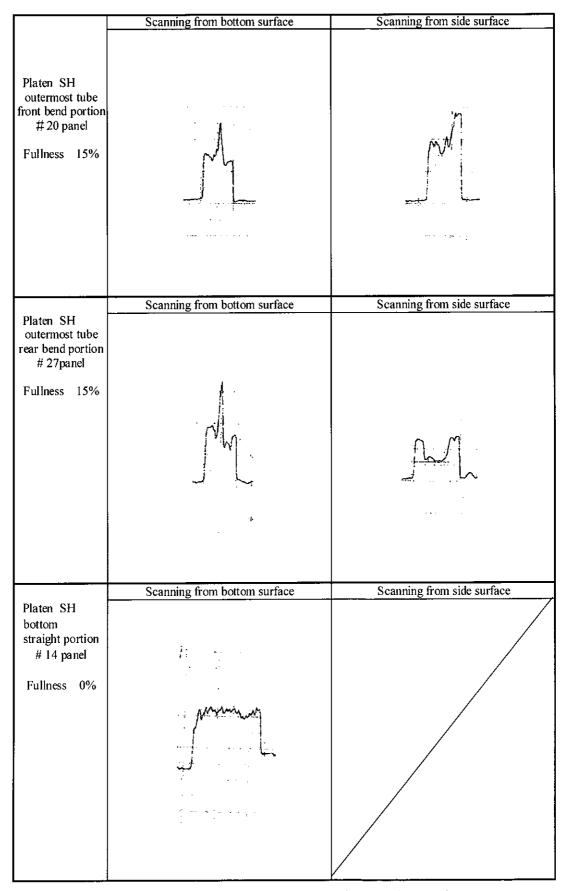
Fig. II-3 Representative deposition signal for this inspection
