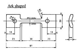
Fig I -26 Shape of creep rupture test specimens
