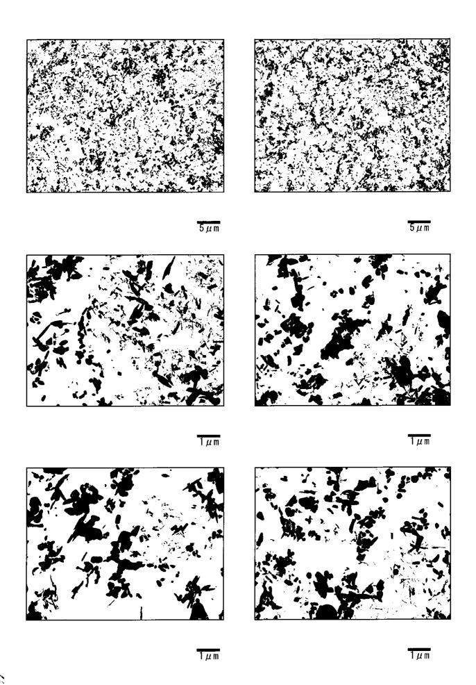
Photo I -4-15 Precipitates by TEM (Transmission electron microscope) observation Platen SH Outlet Header-Left (Circumferential weld at left side: Fine grain HAZ)
