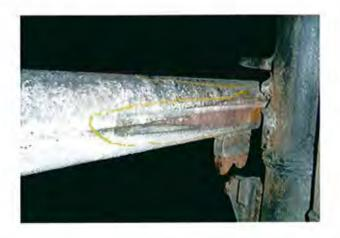
Attrition of cooling spacer tube [extracted Table I -12]
