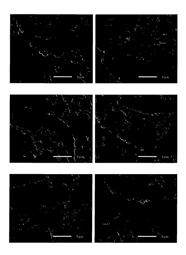
Photo I -5-10 Precipitates along grain boundary by SEM observation De-Superheater-Left (Circumferential weld: Fine grain HAZ)
