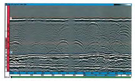
Fig. I -8 X=600~900mm TOFD detection results
