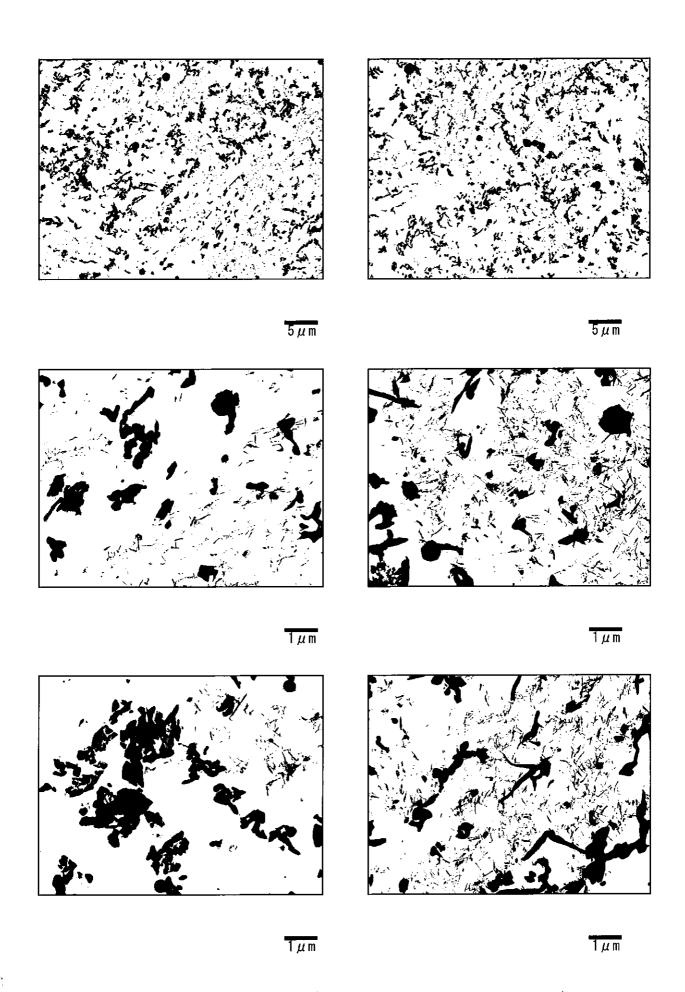
Photo I -4-17 Precipitates by TEM (Transmission electron microscope) observation Platen SH Outlet Header-Left(Circumferential weld at left side: Weld metal)
