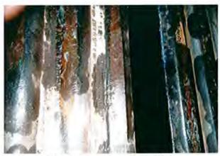
Erosion of front wall tube (extracted from Table I-12)
