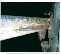
Thining portion of cooling spacer tube
