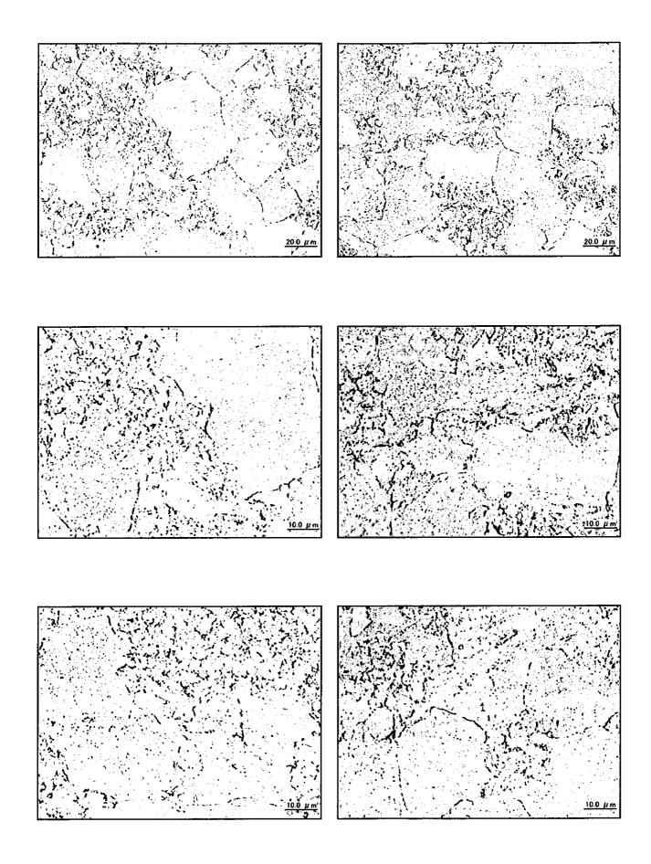
$Photo\ I\ -4-3\quad Microstructure\ observation$  Platen SH Outlet Header-Left (Circumferential weld at left side : Intercritical zone )
