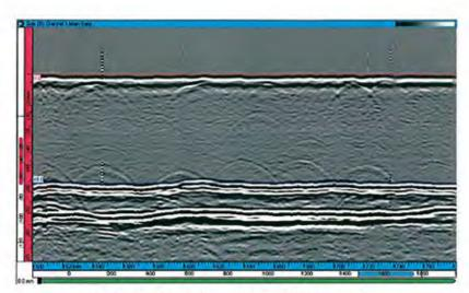
Fig. I -10  $X=1500\sim1780$ mm TOFD detection
