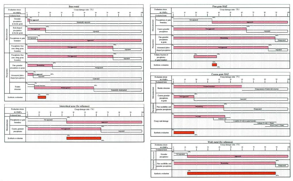
Evaluation Results I -1-2 Platen SH Outlet Header-Left circumferential weld at left side
