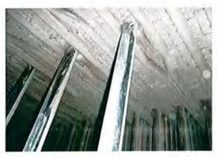
Erosion of rear wall screen tubes [extracted Table I -12]
