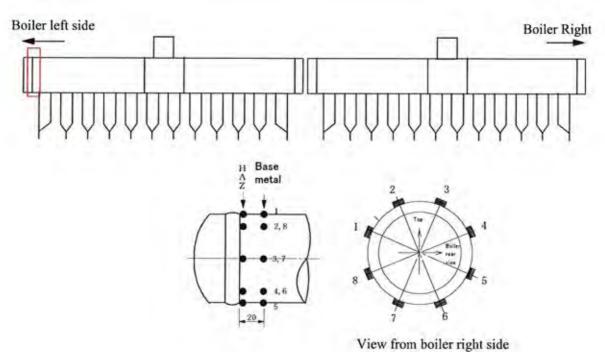
Table I -20 (Singrauli) De-Superheater Pipe Outside Diameter Measurement Results
