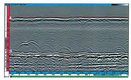
Fig. I -9  $X=1200\sim1500$ mm TOFD detection results
