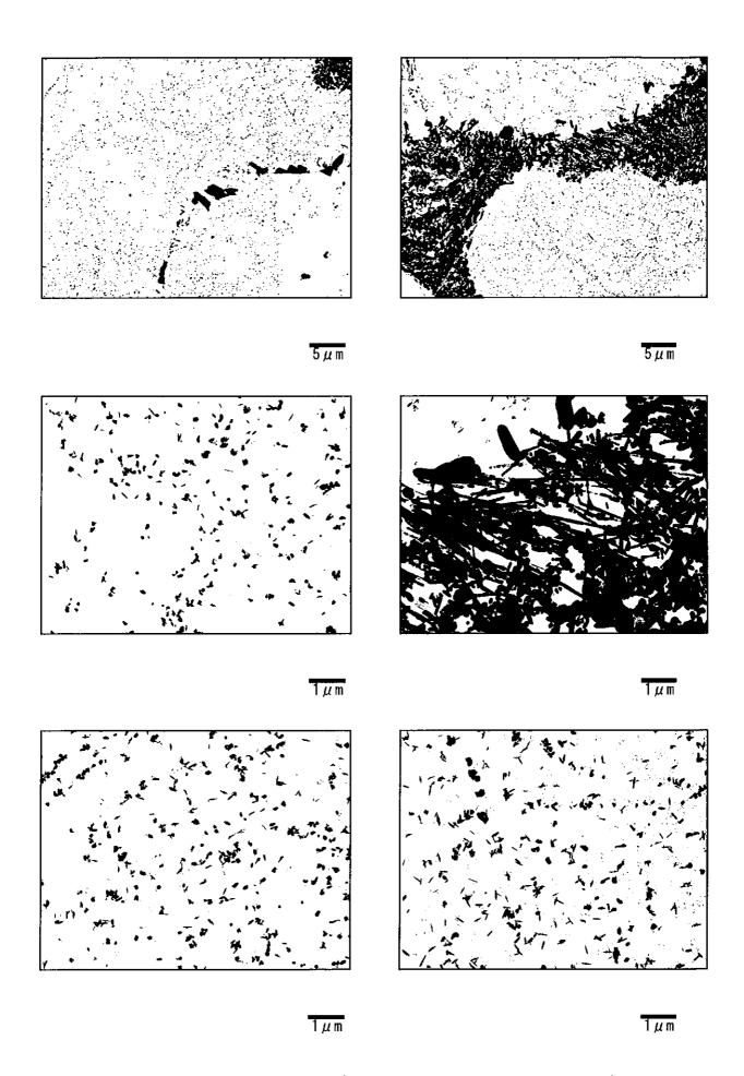
Photo I -5-11 Precipitates by TEM (Transmission electron microscope) observation De-Superheater-Left(Circumferential weld: Base metal)
