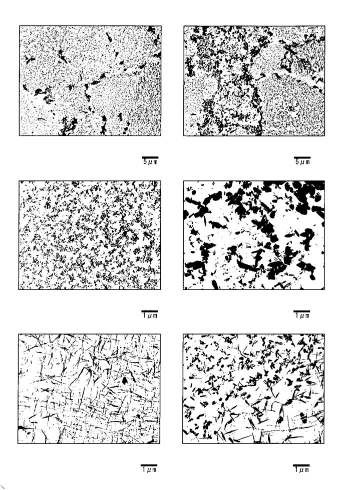
Photo I -4-13 Precipitates by TEM (Transmission electron microscope) observation Platen SH Outlet Header-Left (Base metal at left side: Base metal)
