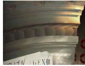
Example (Wear due to Scale)
