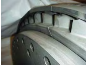
Example (Wear due to Scale)
