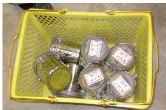
Fig. 6.13-3 Fly Ash Sampling Storage Bin
