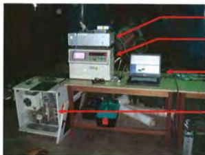
Photo-20 Helium Detection position (Pressure gauge position for #6B vacuum pump inlet)
