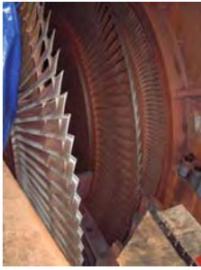
Unit 4 LP Last Blade - Stellite
