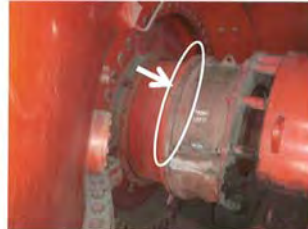
Photo-3: LP turbine packingland Turbine side (Lower/Left)
