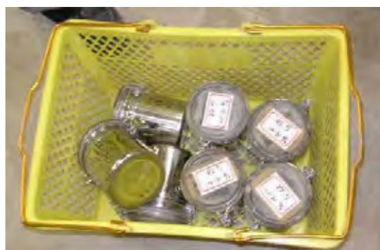
Fig. 6.13-3 Fly Ash Sampling Storage Bin
