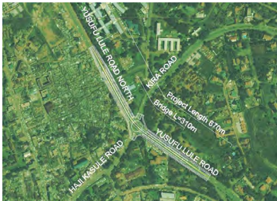
Figure A3.2.37 Existing Condition of Roundabout and Alignment of Planned Flyover
