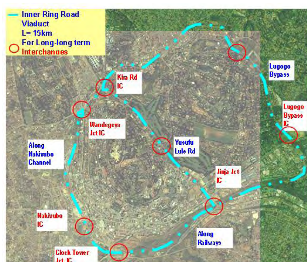
Figure A3.2.48 Inner Ring Viaduct Plan for Urban Motorway Network in Long Long-Term
