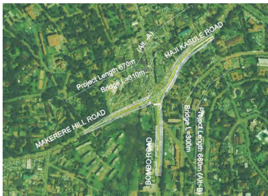
Figure A3.2.42 Proposed Plan of Wandegeya Jct Flyover (Alternatives A and B)
