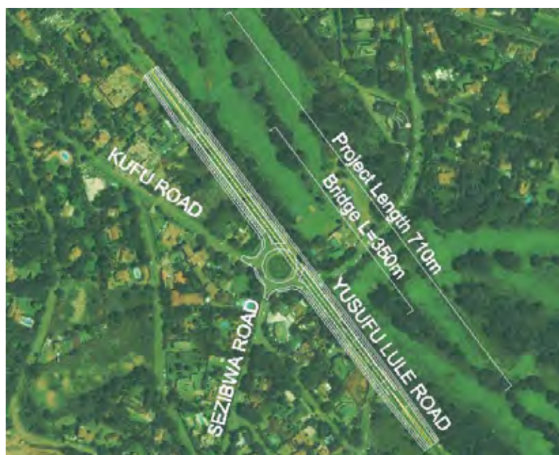
Figure A3.2.39 Alignment of Proposed Flyover (Alternative 1: Long-Term Plan)
