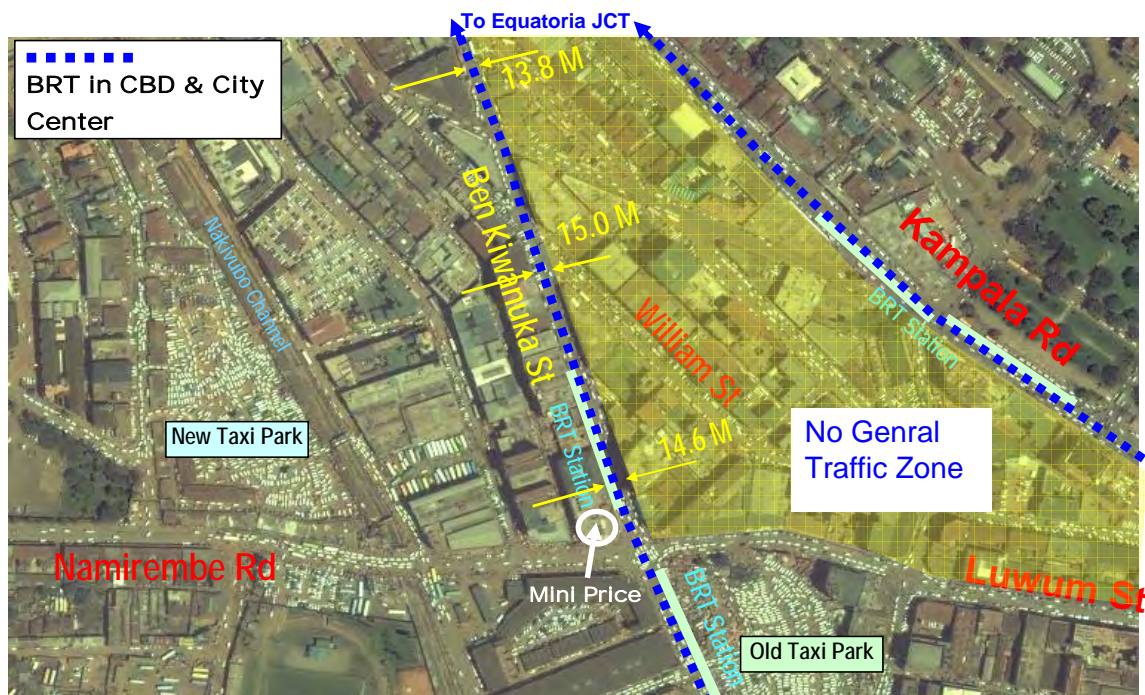
Figure 6.5.6 ROW Width at Ben Kiwanuka Street and Location of BRT Stations
