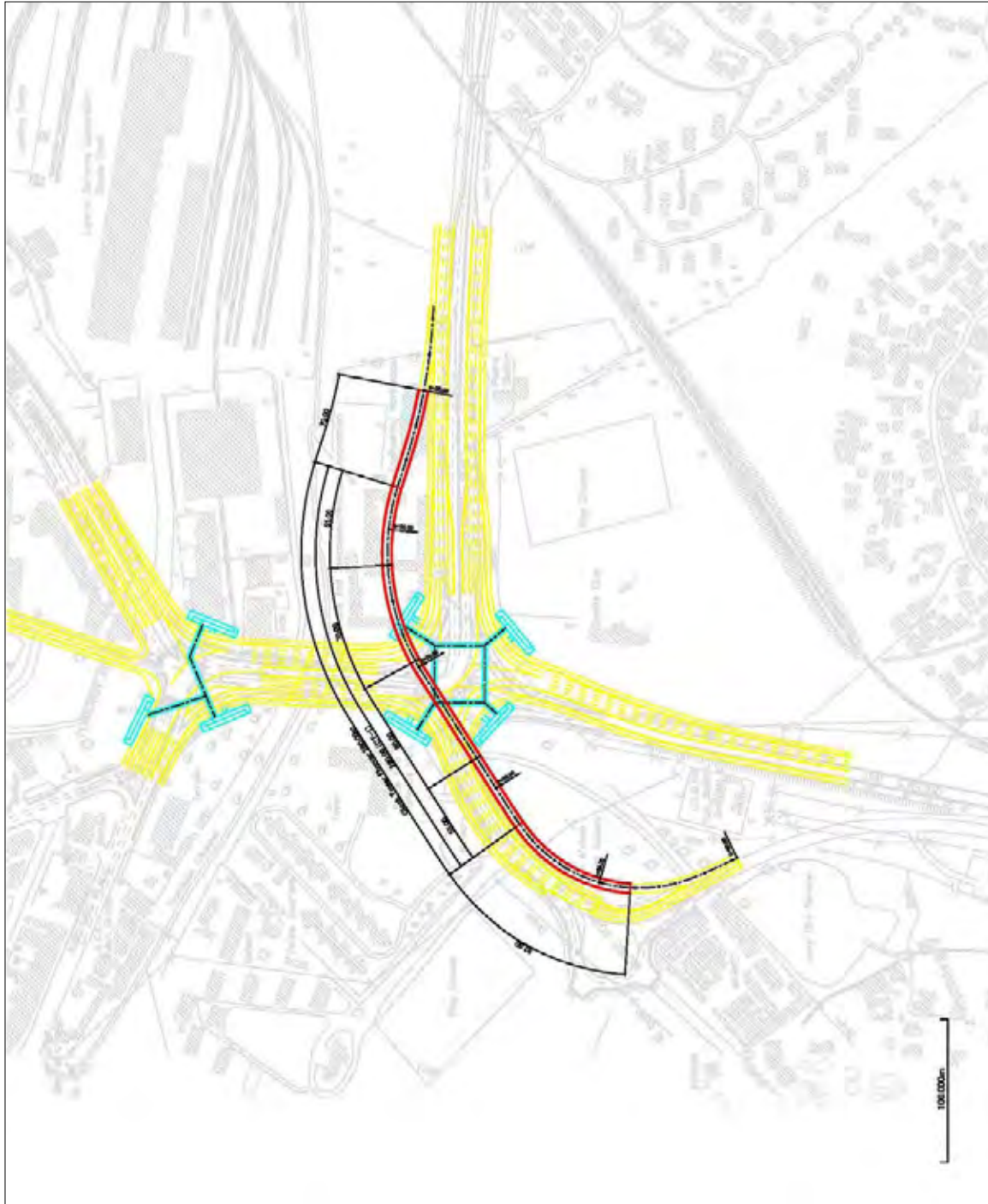
Figure 7.4.9 Preliminary Flyover Plan of Clock Tower Junction
