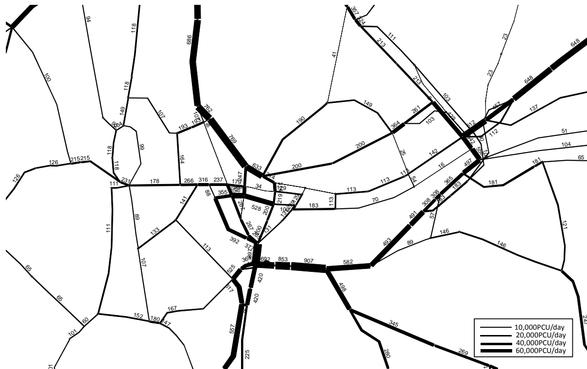
Figure 5.3.10 Result of Future Traffic Assignment at City Center (2023)
