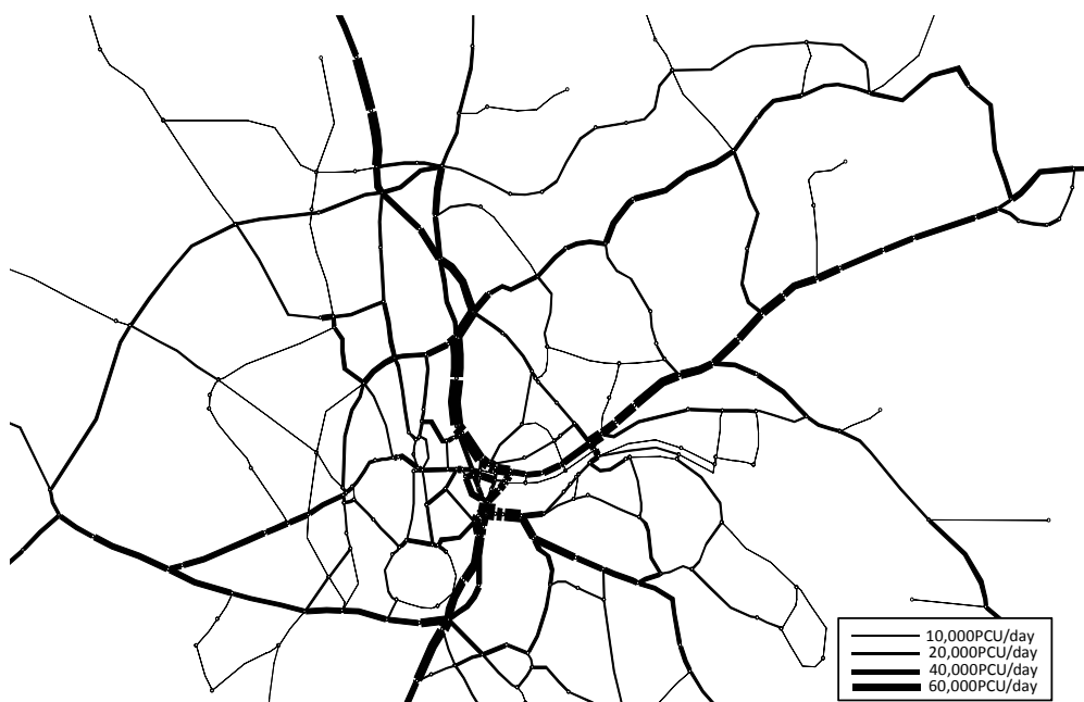
Figure 5.3.4 Result of Present Traffic Volume estimated by Assignment Model
