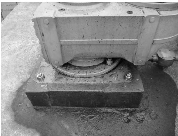
Figure 3.2.42 Grease trickling out
