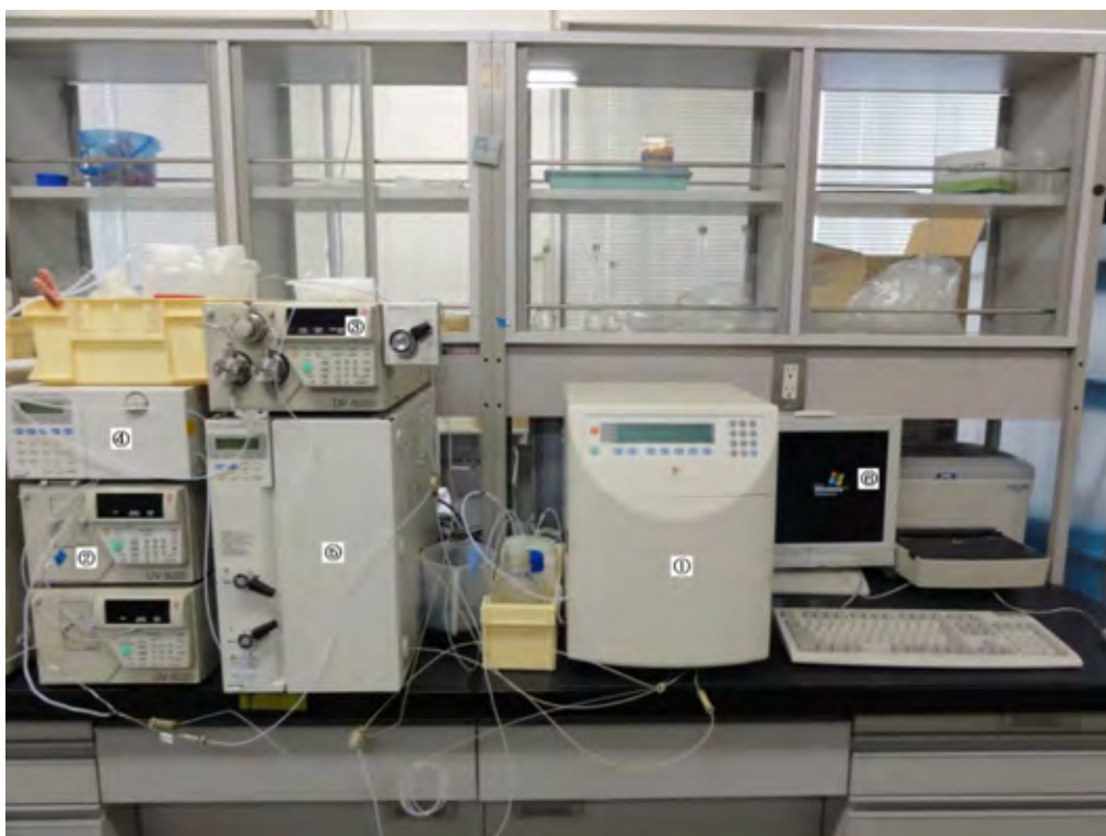
Fig. 4.3.19 Versatile ion chromatograph equipped with conductivity and visible detectors used for monitoring common anions, cations, nutrients, and alkalinity
