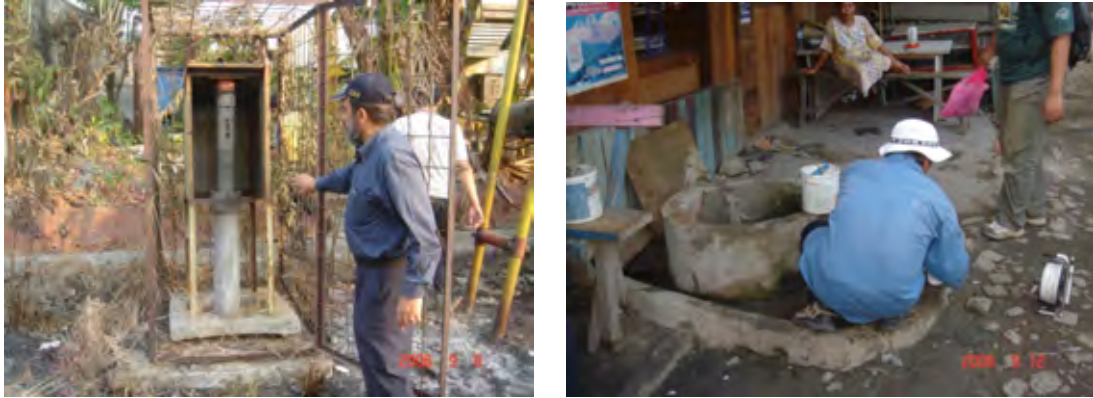
Fig. 5.4.7 Land subsidence monitoring using stand pipe and dug well in Jakarta
