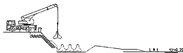
Placement of Blocks from Land Side
