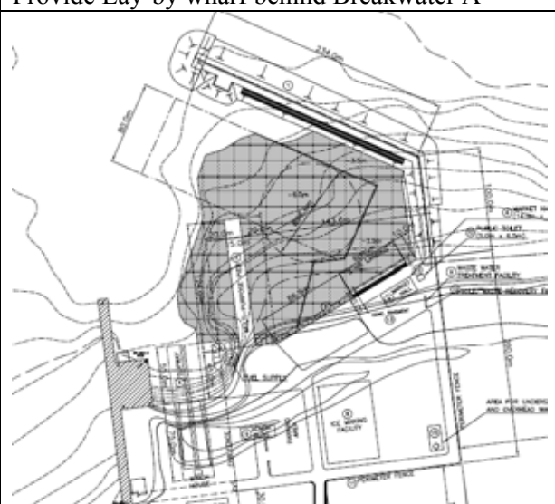
Final Plan showing Location of New Pier, Slipway, Dredging areas, etc
