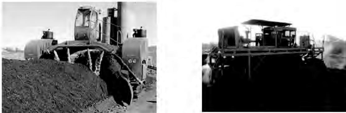
Figure 9. Image of The Windrow Turner
