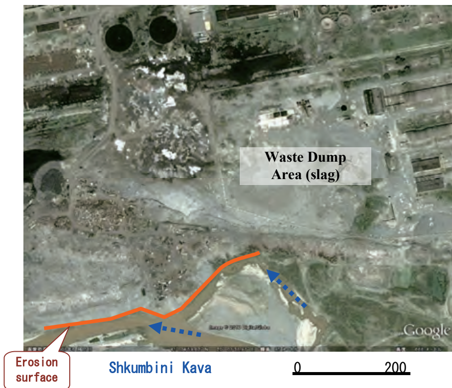
Figure 5.7.2 Present condition of waste dump area (slag) for iron foundry
