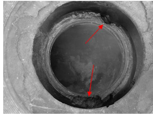
Picture 2: Cavitation erosion (2)
