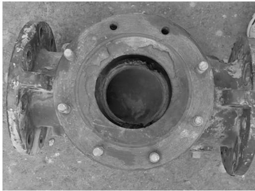
Picture 1: Cavitation erosion (1)
