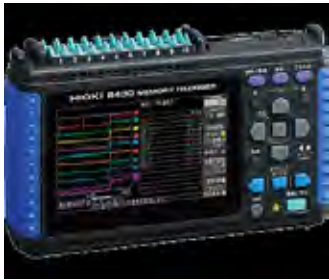
Data Logger for Ampere and Pressure Measurement
