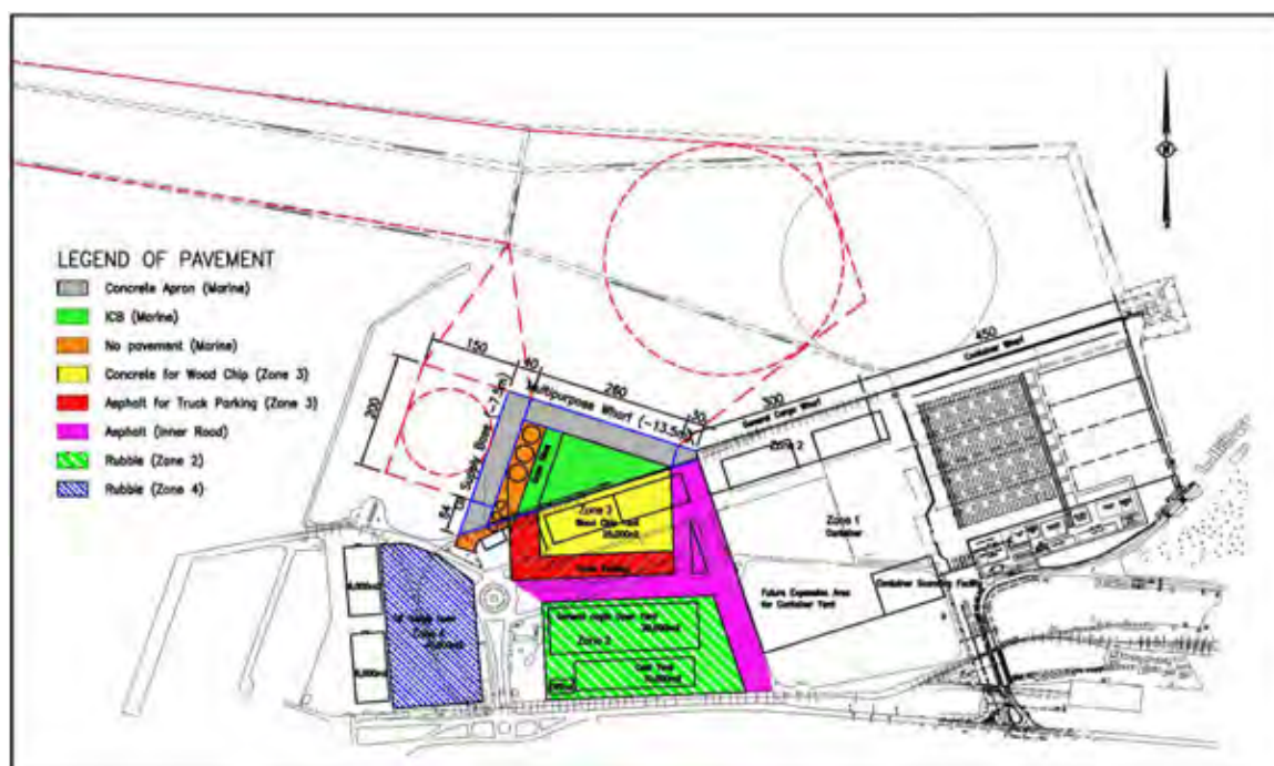
Figure 2.3.7 Layout of Existing Facilities and Planned Multipurpose Terminal
