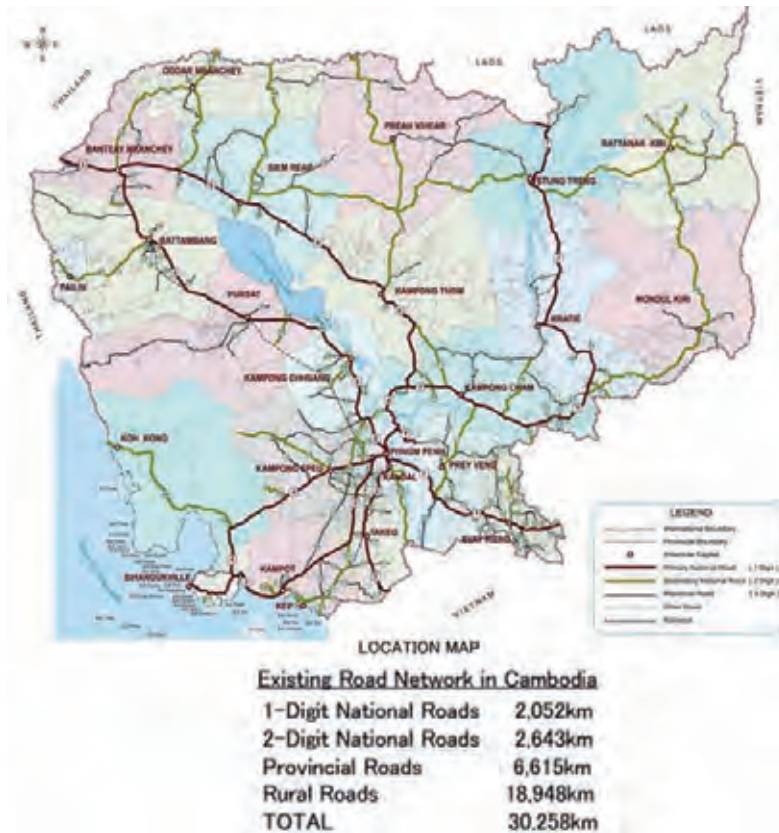
Fig. 2.8.2 Existing Road Network
