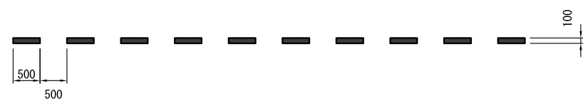
SIDE LINE ② (SHORT BROKEN WHITE) S=1:100
