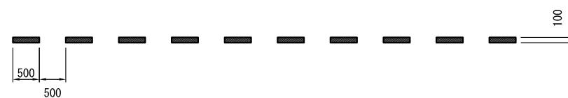
SIDE LINE ② (SHORT BROKEN WHITE) S=1:100
